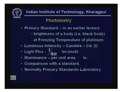
Now in a last class we did look at what should be a primary standard as far as this goes which went through series of changes beginning with the wax candle and Pentium lamp. Finally the primary standard was adapted as the array, a good radiator whose is maintained at the freezing
