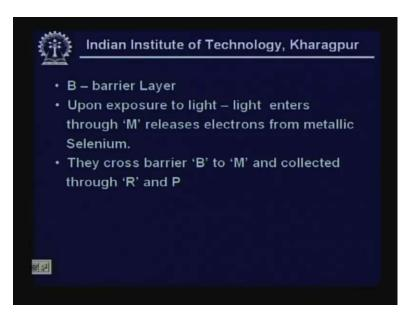
B is the barrier, on exposure to light- light enters through M releases electrons from selenium. They cross the barrier B to M and are collected through R and P. Now once the current is allowed to flow, this current is indicated in the ammeter which could be a micro ammeter and this gives the calibrated in lumens or lux. So that is the principle behind the photo electric cell, this is very important.
