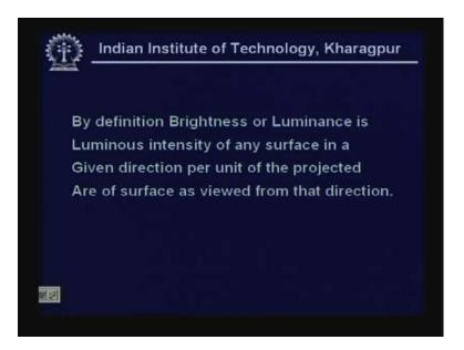
By definition brightness or in fact brightness is also known as luminance whereas the effect we call in terms of illuminance, luminous intensity of any surface in a given direction per unit of the projected area of the surface as viewed from that direction. This is very important in interpreting the light flux diagram in these sources.
