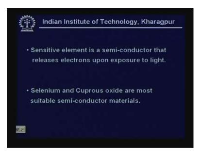
So the first thing is the sensitive element which is a semiconductor which gives rise to electrons or goes into conduction mode on exposure to light. The two materials that have been found suitable for this particular application have been selenium and cuprous oxide, these are the semiconductor materials.
