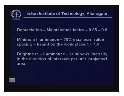
The some factors which are necessary in order to evaluate, there are one major factor is what we called depreciation or known as maintenance factor. In fact depending on the type of maintenance possible or carried out, we can say that if the virgin lamp has a certain light flux radiation capability, it reduces the time and this even for the best of the lamps is around 0.85 which can be as low as 0.6. Then the other thing which is often kept in mind is minimum
