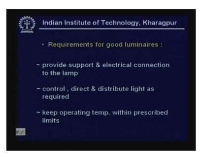
Requirements for good luminaires can be therefore listed as they should provide good support and electrical connection to the lamp, of course depending on the voltage operation. And in fact though I say it should control direct and distribute as required, it's an order to say that these days there are electrical controls available which are part of the luminaire and keeping the temperatures within the prescribed limit. (Refer Slide Time: 00:46:10 min)
