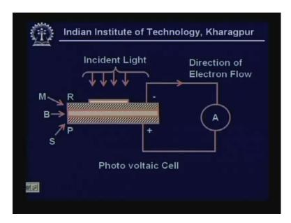
Now it is time to look at the photo voltaic cell. I talked you about that there is a photo voltaic cell. We have what is it called the, it uses the photo electric effect. As can be seen there are three layers, it appears to the three layers but it essentially there is a small thin semi conducting layer S, a small gap on top of which a transparent thin metallic layer M is placed. This gap is talked
