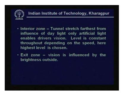
This is the tunnel stretch what we call interior zone which is the farthest from the influence of day light and entirely by the artificial light driver is guided and it is kept constant and usually the highest level is chosen here. Again this is a zone where influence of the brightness from outside begins to appear because he is about to come out.
