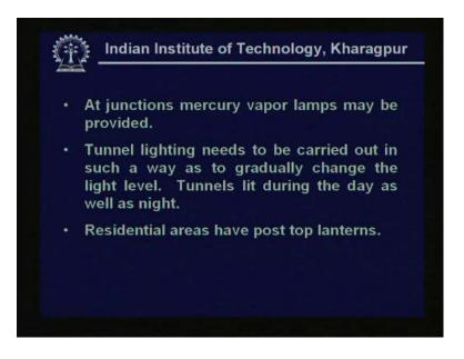
However care is taken at junctions, curves where the intensity levels are increased, mercury vapour lamps are provided. Tunnel lighting is one area which needs special care, it should gradually change the light level and they need to be lit during night as well as day. The post top lanterns which are also ornamental are useful in the residential areas because they do serve the pedestrians.
