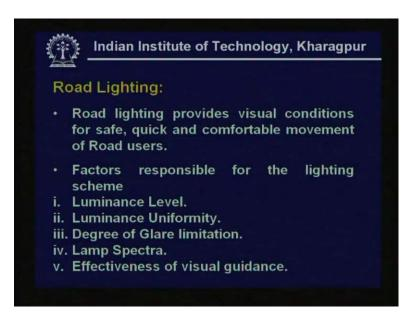
The road lighting actually aims at providing good visual conditions for a safe, quick and comfortable movement of road users. Road users consist of vehicular movement and depending
