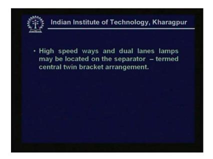
As against this in high speed ways and dual lanes where separators are available, the lamps are located on the separator. So, in very high speed ways and multi-lane roads where separators are there, they are located on the separator. This arrangement is known as central twin bracket arrangement.
