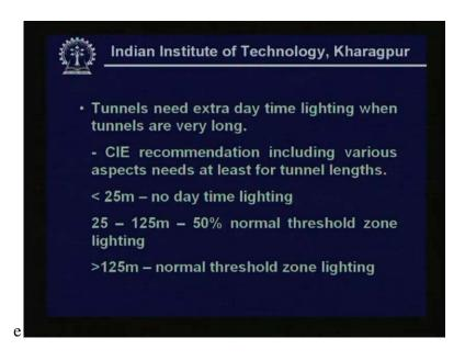
So this is the four zones which are there in tunnels and it must be mentioned that in view of bright light during the day time outside, tunnels need extra day time lighting more so when the tunnel stretch is very long.
