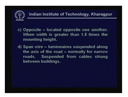
Opposite, located opposite to one another in the wider roads like a venues, when width is greater than 1.5 times the mounting height, we locate lamps on the opposite sides or a fourth arrangement is the what we call as a span wire arrangements basically suspended, luminaires are suspended along the access of the road and this practice is only for small narrow roads where the lamps are suspended on cables or strings strung between the buildings.
