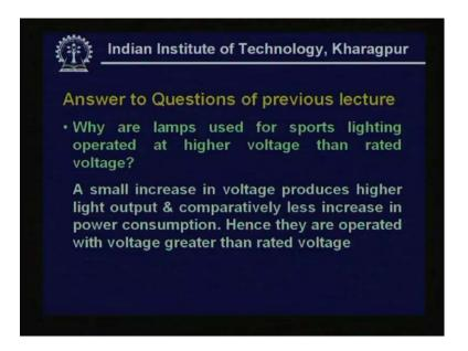
Why are lamps used for sports lighting operated at higher voltage than rated voltage? A small increase in voltage produces higher light output and comparative less increase in power consumption. Hence they are operated with voltage slightly greater than the rated voltage for sports applications. Thank you.
