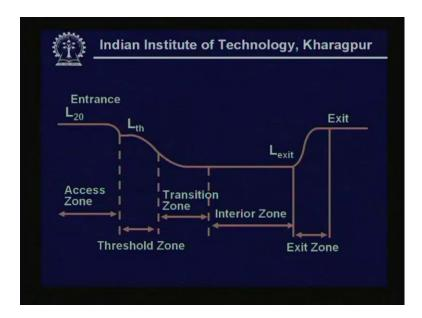
And this is shown in the form a picture, what you are seeing at the entrance is the luminance due to a broad day light and this is a threshold zone and transition zone, interior zone what we are calling is the stretch, the longest stretch or stretch of the tunnel which is very important.
