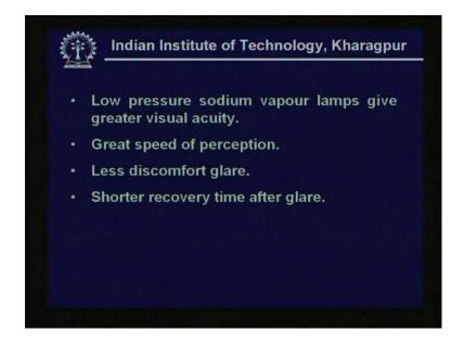
But we find that from the usual utilization point of view, we have already seen the sodium pressure lamps give good performance and is in fact extensively used road lighting lamps. They are known to give greater visual acuity with greater speed of perception and less discomfort glare. The other issue is that subsequent to the discomfort due to a glare, the recovery time for the eyes to become comfortable it's observed that they have shorter recovery time after glare.
