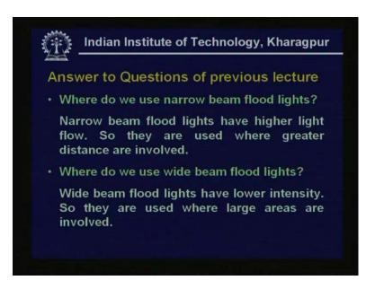
Now taking answers to some of the questions addressed in the previous. Where do we use narrow beam flood lights? Narrow beam flood lights have higher light flows, so they are used where great distances are involved where the mounting height is high. Where do we use wide beam flood lights? The wide beam flood sights have lower intensity; they are used where large areas are involved.
