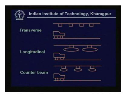
So the picture here shows transverse perpendicular to the plane of paper, the fluorescent lamps are located that's what in the top picture. Longitudinal, they are located along the axis, the spacing can be larger. Counter beam opposite to the traffic flow, so the traffic is flowing from left to right and therefore this presupposes traffic is flowing only in one direction.
