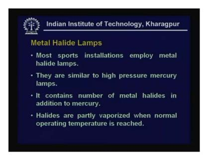
Now as already mentioned most of these lighting installations employ the metal halide lamps. The most sports installations employ metal halide lamps. What do they work on? They are in fact nothing but high pressure mercury lamps, we have said high pressure mercury lamps radiate give rise to the radiation as a band radiation and therefore colour rendering is poor. The number of metal halides are added in addition to the mercury vapor to improve the colour, colour rendering.
