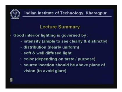
In effect what we have seen in this lecture is that good interior lighting is governed by intensity that's ample to see clearly and distinctly, creating nearly uniform distribution which is soft and well diffused light. Colour of course depending on the purpose and taste, keeping the sources well above the plane of vision to avoid glare.
