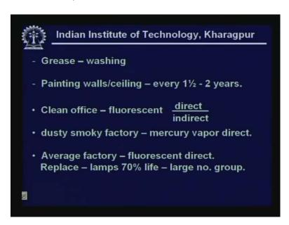
Grease should be washed and that is as for the lamps but the interior, that is a walls and ceiling are preferably painted every one and half to two years to create. With all this the offices interiors could have floors and lamps with direct or indirect luminaries. The dusty, smoky, factory environments could have mercury vapor lamps with direct luminaire and average factory could
