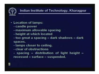
Having said all this, the next thing that comes is the location of the lamps that depends on the candle power. The maximum allowable spacing between the lamps, the height at which to be located. Remember too large spacing would involve what is called dark shadows or dark space between. Remember the aim is to locate have as uniform lighting as possible, lamps best fitted
