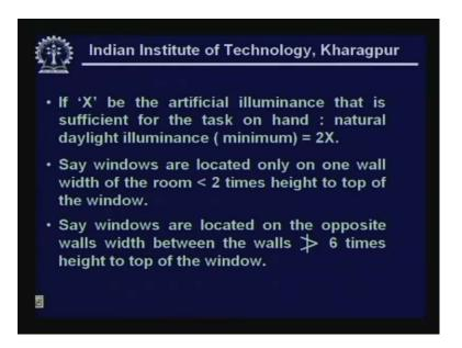
On the other hand if the windows are located on opposite walls, the width between the walls should not be greater than 6 times the height to the top of the window. Going with the same argument, if the top of the window is around 5 feet, 6 times that would be 30 feet, so it should be less than 30 feet between the two walls. These are some of the guidelines.
