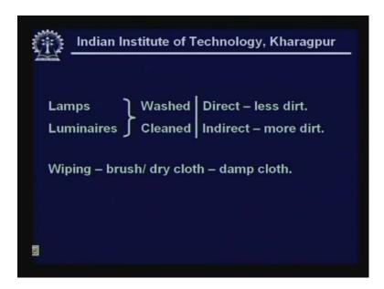
The lamps and luminaries need to be maintained, luminaries they could be washed, cleaned. In direct case there is less dirt, in indirect case there is more dirt so there is more periodic requirements. This could be wiped with brush or dry cloth or damp cloth.
