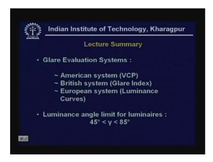
Glare evaluation systems comprise of American system which is visual compare percentage, British system which talks about glare index based on the zone of illumination and the most prevalent European system is luminance limit curves. Luminance curve limit looks for luminance angle between 45 to 85 and based on the curves one evaluates the glare.
