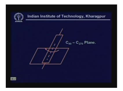
As opposed to this there could be a plane where we will constitute that is  $C_{90}$  to  $C_{270}$  plane that is perpendicular to the length of the axis. So we have the critical angle which should be I mean the zone of the thing between 45 to 180, 45 to 85 and we also look at the type whether it has luminous sides or not or sides are not effective then the orientation whether along the axis or perpendicular to the axis then one can look at the requirements.
