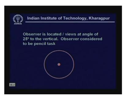
And this is what we called task visibility. Now this is best, this is believed is best when observer views at an angle of 25 degrees to the vertical and this is considering one is looking at a task is basically this circle with the dot shows that angle and observer is considered to be viewing a pencil task in fact it is believed that is the it is the most tenuous thing to look at a pencil task.
