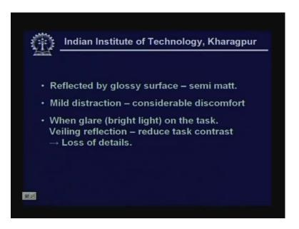
These when they are reflected by a glassy surface or a semi matt surface, they become very important but one must say with all this, there is a mild distraction which creates discomfort but it does not really what you call cause any damage or discomfort to the eye. The glare if it is on the task, one has to look at the contrast and see that there are no loss of details.
