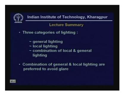
Three categories of lighting are important that in general lighting, local lighting and combination so that an appropriate glare is avoided. In fact a suitable combination of general and local reduces glare to a very large extent.
