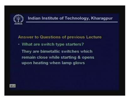
What are switch type starters? They are bimetallic switches which are very commonly used, remain closed while starting and opens upon heating when lamp glows. Thank you.
