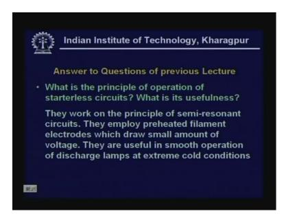
What is the principle of operation of starterless circuits, what is its usefulness? They work on the principle of semi resonant circuits, they employ preheated element filament electrodes which draw small amount of voltage. They are useful in smooth operation of discharge lamps at extreme cold conditions.
