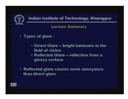
The types of glare are direct glare, when the bright luminaire is in the field of vision, reflected glare when it is reflected from a glassy surface. Reflected glare causes more annoyance than direct glare though not harmful it creates interference.
