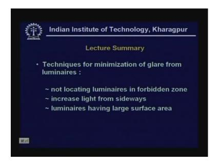
Techniques for minimization of glare from luminaires never locate them in forbidden zone, increase the light from sides and employ low luminaires but large surface area luminaires.
