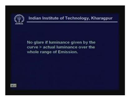
And if we find that illuminance given by the curve not illuminance, luminance given by the curve is greater than the actual luminance then we say it is glare free. Obviously it means the source in the zone of illumination or zone of eye, eye zone is not going to be very bright and therefore it is glare free.
