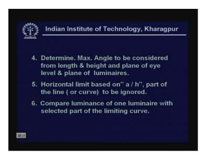
Once we select the curve we determine the maximum angle. Recall the diagram where we saw gamma max based on the length of the illumination plane and height of this plane from the eye level and we consider only that portion of the curve which is above 45 upto gamma max then compare this with the luminance curve obtained for a light system.
