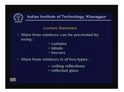
Glare from windows is always prevented by using curtains, blinds, louvers is of two types, there could be reflected and veiling reflections that is light trying to percolate in between the curtains or blinds.
