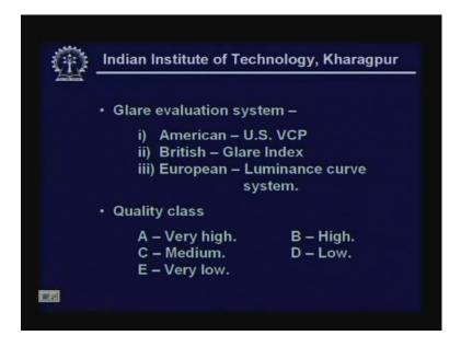
So glare evaluation system as we see is one American which basically is VCP or visual comfort percentage. The British system is the glare index, the European is the luminance curve system and all this requires to consider the quality class. A corresponding to very high quality lighting, B corresponding to high quality lighting, C is the medium quality, D is the low quality and E is very low.
