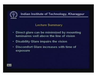
Direct glare is minimized by mounting luminaires well above the line of vision. Disability glare is what impairs the vision which happens very rarely, discomfort glare increases with the time of exposure and one is relieved after a period of rest.
