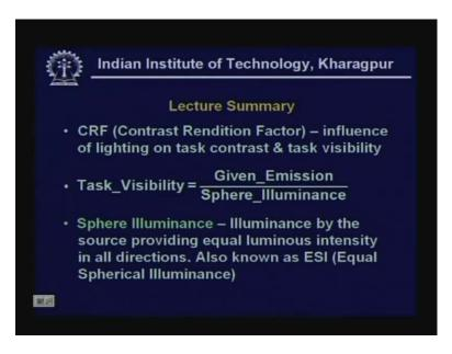
Contrast rendition factor influence lighting on task contrast and task visibility which is defined as the given emission to the sphere illuminance and sphere illuminance being the source providing equal luminous intensity in all directions ESI.
