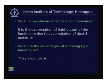
What is a maintenance factor of a luminaire? It is the depreciation of light output of the luminaire due to accumulation of dust and moisture and age. Advantage of using diffusing type of luminaire? They avoid glare. Thank you.
