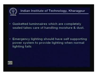
And wherever moisture is involved gasket should be provided and completely shield so that dust or moisture does not take place. Now for the sake of having different emergency lighting or safety lighting, one should have self-supporting power system when normal lighting fails. (Refer Slide Time: 00:52:21 min)
