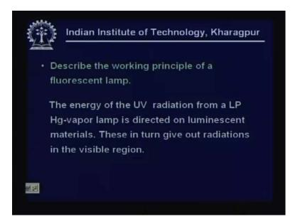
Working principle of a fluorescent lamp? The energy of the UV radiation from a low pressure mercury vapour lamp is directed on luminescent materials or phosphors; these in turn give out radiation in the visible zone.
