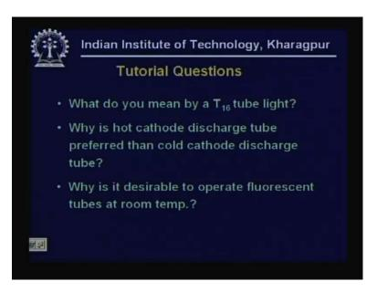
What do you mean by a  $T_{16}$  tube light, why is hot cathode discharge tube preferred? These are some of the tutorial questions that can be addressed from this lecture preferred than cold cathode discharge tube. Why is it desirable to operate fluorescent tubes at room temperature?
