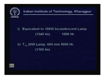
This is equivalent to a 100 watt incandescent lamp and it can have whereas an incandescent lamp has only 1000 hours of burning life whereas that would be comparable to a 20 watt lamp which has about 5000 hours of convention. So this is the comparison one could have for an 18 watt CFL.
