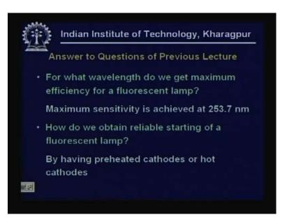
For what wave length do we get maximum efficiency of a fluorescent lamp? The maximum sensitivity is around 253.7 nanometers. How do we obtain reliable starting of a fluorescent lamp? By having preheated cathodes or hot cathodes.
