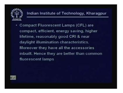
CFLs are compact efficient energy saving and have life time but reasonably good colour rendering I said colour rendering is not so good. All the accessories are in built and therefore they are usable in the conventional lamp holders where incandescent lamps were employed.
