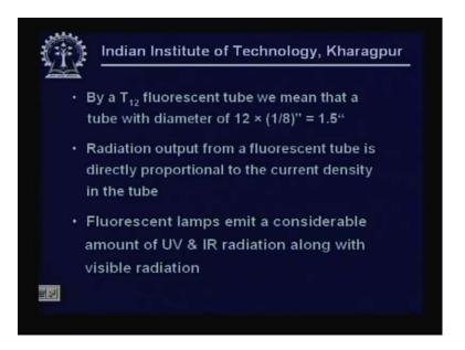
By a  $T_{12}$  we mean that it's got a diameter of one and half inch radiation output from a fluorescent lamp is proportional to the current density in the tube. This fluorescent lamp emits considerable amount of UV and IR radiation along with visible radiation and UV radiation is beneficial in small quantities.
