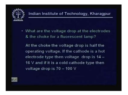
What are the voltage drop at the electrodes and the choke for a fluorescent lamp? At the choke the voltage drop is half the operating voltage of the cathode is a hot electrode type then the voltage drop is around 14 to 16 and if it is a cold cathode type it's around 70 to 100 volts. Thank you.
