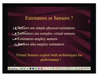
So, the question is the same, in a sense now that we understand estimation, we know that estimation is basically the computation of one quantity from another quantity, using a model right; so odd sensors very rudimentary estimation. So for example, sensors are simple physical estimators. So, you actually sense the resistance change and from that, you can estimate the temperature, right.
