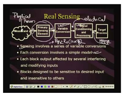
For measurement, we typically the first thing that is used, is called an a is called as sensor, typically it is called as sensor. So it is a device, so what does it do? This picture discusses that. So, so here we have some Measurand; which is a which is a which is a which is a physical process, so it is a physical process may be it. We are we are we are interested in measuring, some temperature pressure, strain, whatever.
