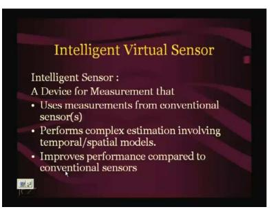
So, I will keep this slide, so an so an intelligent virtual sensor is nothing but a device; that makes a measurement from number of, could be a possible a number of conventional sensors, employs an estimation algorithm and improves performance compared to conventional sensors. (Refer Slide Time: 12:34)
