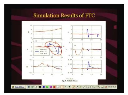
So, this is the this is actually, this actuator was made a part of a full missile model; and then we wanted to see, that if such a fault occurs in the actuator then what happens to the missile. And it turns out that, you see without the fault tolerance control the the signals, that are they are they are actually quietly differ from, what the desire levels of signal should be.
