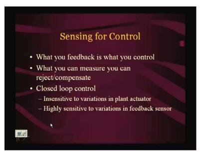
Remember, that what your feedback is what you control. So, in a control loop, if you add a one volt bias to the to the sensor then if there is bias or if there is any kind of noise in sensor; exactly the same type of noise will actually appear at the output. So, the so so the control system is actually, traditionally, a lot robust with respect to the forward path element characteristic.
