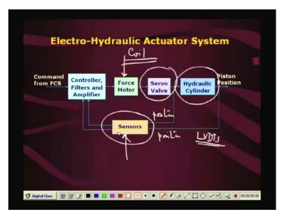
So, this is the block diagram of that actuator system which is electro hydraulic; in the sense that, in the sense that you have this is a hydraulic servo valve, this is the hydraulic power piston. So, using, these are the sensors which sense position, the servo valve full position and the piston ram position, they are basically LVDTs. So, they gave the feedback to the controllers and the controller drives; what is known as the which is which is nothing but a coil.
