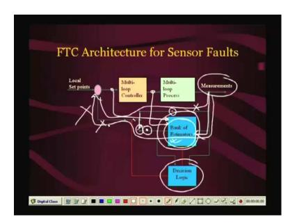
So, the sensor is actually feeding back signal like this. Now, if it is faulty, if it is faulty if there is any fault here; suddenly this loop path will be broken, it will be broken and this will become open loop. They will completely destroy the control. So rather than that, if we have a bank of estimators, this could be Kalman filter, there could be observers, there could be artificial neural networks, there could be various kinds of models which will estimate this quantities.
