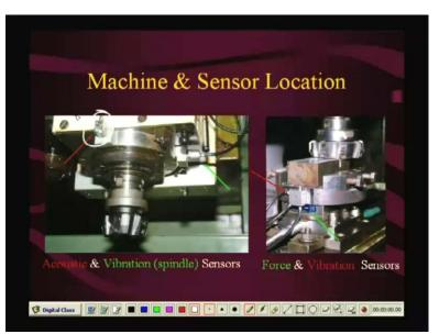
So, these are you know, some of the point some of the points, we actually put the physical sensors. So, you have an acoustic sensor here which is which, senses very high frequency internal vibration, you should cracks etcetera, inside the thing. We did not we are not going to talk about that too much.
