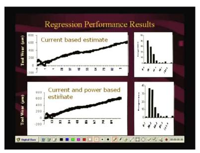
Similarly, again the the advantage of having sensor fusion in terms of accuracy is shown. So, you have current based estimates here, here you have current and power based estimates. So, it turns out that the current and power based estimates are somewhat, straightly not much; but still somewhat improved over the force based estimates or only current based estimates.
