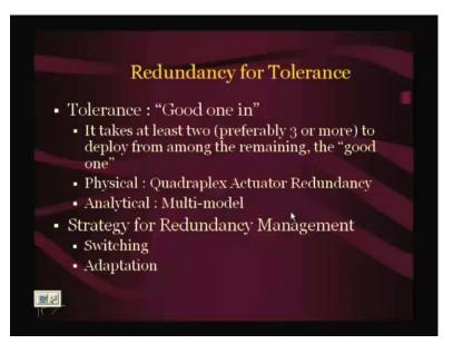
So, similarly while you need redundancy for detection, you also need redundancy for tolerance because tolerance is actually; basically tolerance is bring the good one in, detection is get the get the odd one out, and tolerance is to bring the good one in. So, obviously you you will you will you will have to have a good one and in many cases, it turns out you see, you cannot you can create information from models and computation, but you cannot create energy.
