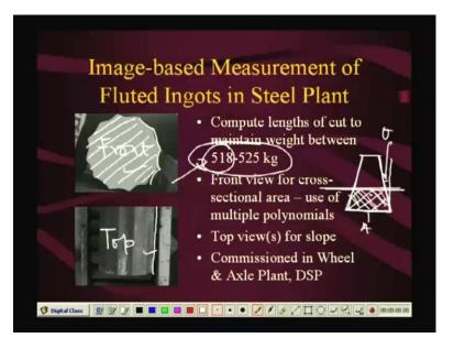
So, for example, let me first start with a very simple example. This is an example where you know, I have been involved with this work; where we were required to, require to measure you know, there is there is a there is a cylindrical ingot which you can see, here in this picture. This is an ingot, it is a it is a cylinder. You can see its cross section; it is actually made of steel. Now, the railway wheels are made out of these ingots, in the Durgapur Steel plant of SAIL.
