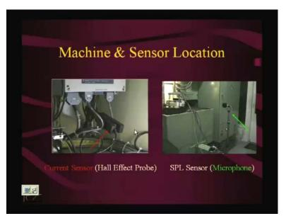
So, we have some current sensors, you know current sensors sensing is very simple, compared to force sensing. So as we shall see that, we can we we wanted to see whether rather than using force sensor, whether we can use a current sensor and then estimate the wear. So, that we can find the technology which is which is implementable much much cheaper than using a force based technology.
