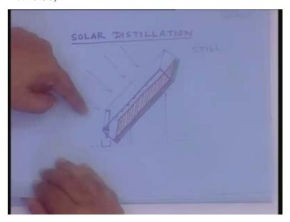
One, like the flat plate, which will have the advantage of, what is the advantage of this? That it can always face the sun which the horizontal design cannot, right. But, the disadvantage is that here you have to have some way of keeping the surface wet all the time, which may not be trivial and here you have the problem of keeping it wet is trivial, you simply have to pour, but it does not face the sun all the time. Obviously, that is the concept of the solar distillation, solar still.
