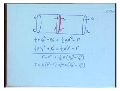
You will have half rho V infinity square plus P infinity is equal to half rho V square plus P plus. Again, we can write the Bernoulli's principle from here to here, right. So, since we will have to do some manipulation here, we will write this one first and this one later. So, we will write it as half rho V 2 square plus P infinity here is equal to half rho V square plus P minus, right. So, having written these two equations, we can subtract this from this
