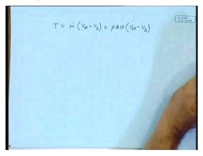
The thrust can also be written as m dot V infinity minus V 2. So, this is, m dot is rho A small v that is the rate at which it is passing. What is the rate of flow? It is through this, right and so, you have rho A small v times V infinity minus V 2.
