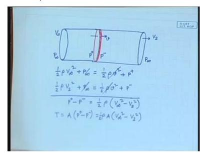
But, you will notice that here we considered some kind of a disc that remains there and extracts energy. Obviously, it does not work on the thrust principle. If it works on thrust principle it would recede, right.
