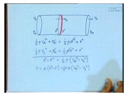
So, where was the picture? Here, which means that the maximum power can be extracted only when the speed when it goes through is two third of V infinity, because it is, it is defined as 1 minus a, fine. So, now we can, we can substitute this here, one third here. So,
