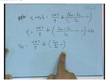
In the last class, we have derived that the open circuit voltage is given by this. This fellow is a constant. Then, the relationship between this and that, obviously this is far larger than this, so 1 can be ignored. So, ln, this fellow is constant, ln of the photo current. Obviously, if the photo current becomes half, how much will the logarithm reduce? So, how much?
