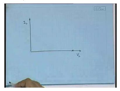
It will have a character. If you draw, you can yourself solve the Newton-Raphson equation and you will get it that is V L here and I L here. You have seen in the last class that if you substitute I L equal to zero, then you will get a specific value of open circuit voltage. So, open circuit voltage at I L zero has a specific value, right.
