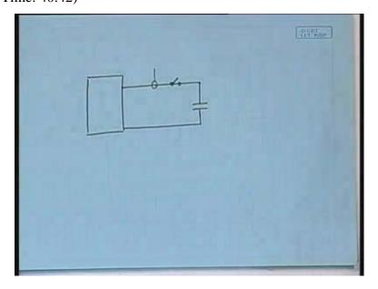
All that you need to do is if you have a photovoltaic panel that will require an online data acquisition system which will measure the current and the voltage, but here you have nothing but a reasonably large capacitor and here your switch. When the switch is open, it is open circuit voltage you get, right. The moment the switch closes, what will be the condition? Across the capacitor, across the capacitor there is no voltage as yet. So, how much current will flow?
