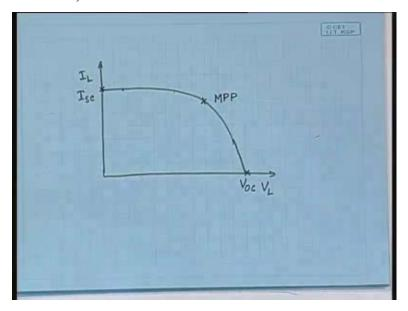
So, there will be a specific value of the short circuit current. In between, what the character will be? In between this character will be of this shape. This shape is essentially the characteristic of the photovoltaic panel. So, this point is V oc and this point is I sc, short circuit current and the open circuit voltage. This is the characteristic; this curve is a characteristic of the panel.
