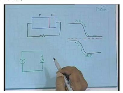
Now, if we have this balance, that means some amount of charge is separated creating the I ph, photocurrent and some of it goes through the diode without going through external
