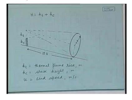
Now, let us look at this. The plume rises to this height and then that expands like a, like a cone and finally it reaches this particular point. So, when it reaches this particular point, so what is the volume flow? We are interested where it touches the ground. That means it has come to this level and now we are interested in the volume flow rate of the pollutant. So, how much should that be? Depends on the area, depends on this flow rate.
