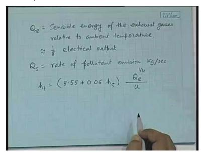
Your, let Q e is the sensible energy of the ... relative to the ambient temperature. Do you have any idea how much it is? It is the energy contained in the flue gas. How much? In general, rough estimate is about one eighth of the electrical power output of the power station. So, this is approximately one eighth of the electrical output. So, one way of
