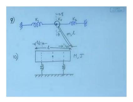
How, about this sum of the clocks, have it like this a spring, another spring, so there are two springs and it is able to move like this and there is a tortional spring that connects a rod. So, this is a tortional spring that also gives a springy effect. So, how will you define in this case, you can say this is k 1, this is this one is k 2 and this is a tortional spring say k r rotational spring and then it has a mass m length l.
