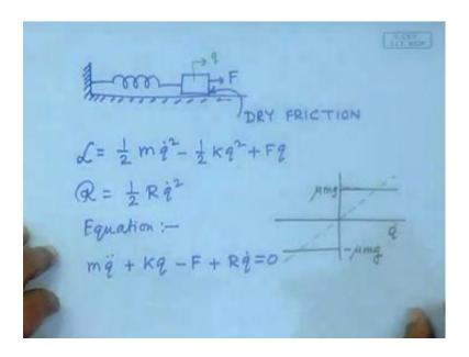
So, let us do a problem with a dry friction element. Suppose, you have surface, there is a spring connected to a mass and where it is pulled with a force F and this fellow is a dry friction. This surface is a dry friction surface. Again, in this case the convenient definition of the state variable would be the q, where q is measured from the unstretched position of the spring that will be convenient.
