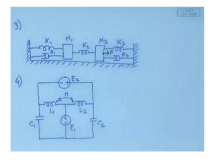
How about this problem 3, there are two masses, this one is connected by a spring damper arrangement. This one is also connected by a spring damper arrangement and these two are connected by means of a spring and say there is a force F, pulling this mass. In that case, how will you define the state variables, again there are two masses; their positions uniquely define the systems, positional status.
