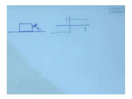
So, where you have got a body resting on a dry surface and if somebody pushes it and then it will initially, it will not move, and then when that threshold force is exceeded, it starts to move and then after that the force due to friction remains more or less constant. So, that is what the character is and we have already seen that, it can be represented by means of a graph something like this, q dot here and a force here.
