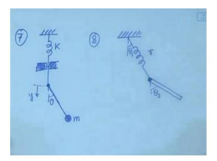
You have got a spring and there is a say guide and this well as coming, so that this is not allowed to move this way, this only allowed moving that way and here you have a point of suspension from which the pendulum is hung. So, this is a guide that allows it to move only up and down. In that case, how many variables would you need, think 2, which 2?
