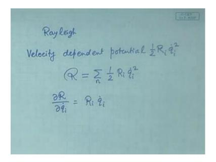
Rayleigh proposed that, this can be done by defining a new type of potential which is obviously velocity dependent. So, velocity dependent potential, potential that would be expressed as half R i q i dot square, along each of these directions. So, total Rayleigh potential is I will express the R Rayleigh potential, in order to distinguish it from this force coefficient R by some kind of a script R. That is equal to summation over a number of generalized coordinates.
