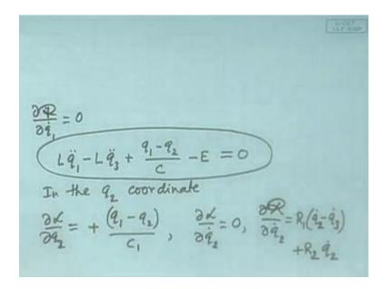
And your Rayleigh function is what is your Rayleigh function, yes it is independent of q 1 0. So, now if you write the equation it will be, so the equation is d d t of this which means L q 1 double dot minus L q 3 double dot. Then this one negative of this one q 1 minus q 2 by C minus E, this term Rayleigh term is 0, therefore this is ok. Let us do it the direction of q 2 also, because that is that illustrates the use of the Rayleigh term.
