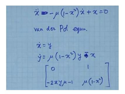
You have say a equation something like this, x double dot is equal to or minus mu 1 minus x square x dot plus x is equal to 0, this equation is actually called van der Pol equation. So, in this case how will you proceed again proceed in the same way, so we will say x dot is equal to y and y dot is equal to mu 1 minus x square x dot is y plus x fine. So, your Jacobian matrix is if you...
