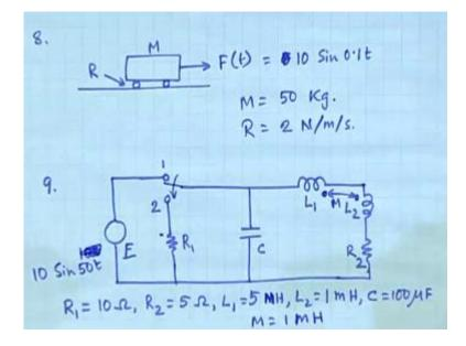
Now, you have a cot which is being pulled with a force F, there is a mass M and here is a friction R. The force is F or I will write number 10 sin 0.1 t. That is, how it is being pulled M is equal to 50 Kg and R is equal to 2 Newton's per meter per second. So, what will happen, here is a sinusoidal forcing, that sinusoidal forcing will make this fellow also sinusoidal move.
