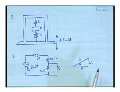
Two, the system is like this, here is R, M, K and this ground is oscillating with A sin omega t. So, obtain the equation for the vibration of this mass, you will see that this arrangement effectively acts as a vibration or isolator. That means, if the this thing is vibrating, then that vibration will not be will be somewhat less in this as seen in the mass.
