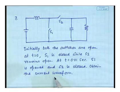
Seven, again a electrical problem you have got a battery, here you have got an inductor, but there is a switch here and there is another switch here. Again initially both the switches are open at t is equal to 0, suppose this is s 1, this is s 2, s 1 is closed while s 2 remains open. At t is equal to 0.01 second s 1 wait, initially s 1 is closed s 2 is opened and then s 1 is opened and s 2 is closed.
