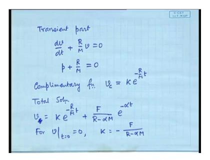
Then, for the transient part you have to take d v d t plus R by M v is equal to 0, what is the characteristic equation, we write this as d v d t as p. So, p plus R by M is equal to 0 that is how we have wrote it, so you have the complimentary function is...
