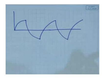
If it is a R C circuit, then what will be the waveform be the capacitor tries to charge to the applied voltage. But, then the applied voltage changes to a negative value it is tries to follow it again it tries to rise it tries to follow. How did I obtain without solving i, simply by understanding, that all the time it is trying to reach the equilibrium point and it has to do, so exponentially. So, all these will be exponential things, there is no other way of for it to do.
