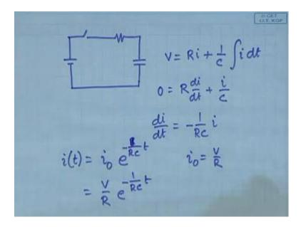
In case of the R C network how will you do that in case of the R C network, again writing the equation first, it will be V is equal to R i plus how much is the current here 1 by C integral i d t how is the voltage here. So, you have you just differentiate it you get 0 is equal to R d i d t plus i by C, so the equation is d i d t is equal to minus 1 by R C times i. Now, in the same way if you obtain the equation you have obtained the solution, it will be i of t is equal to some initial condition.
