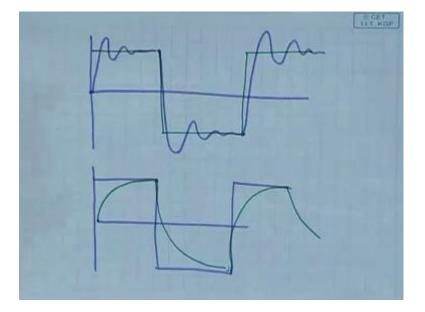
In time domain what will be the behavior like, in time domain how will it look. Suppose, I am drawing the wave form for V C, then it will try to reach V C comes very close and then it jumps. Have you seen this waveform in your experiment on the C R O, on the R L C circuit.
