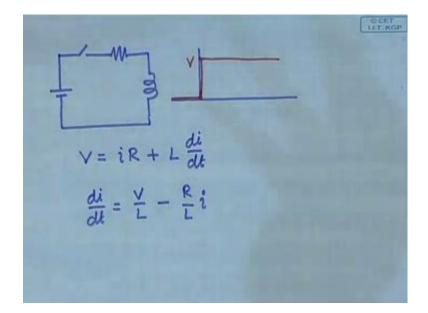
So, if you have a, let us take an example circuit for example, if you have a circuit something like this a battery here connected with a switch to a R L circuit. So, if this the switch is closed the applied voltage will be what, it was earlier 0 at this point it will rise to some value and then it will be like this. So, the applied voltage on this R L block will be initially 0 and then at some point it will be applied.
