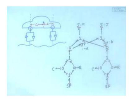
Imagine there is a car and as this car I will not draw the wheels, because the wheels are actually suspended. The car is suspended on the wheels by means of a suspension which is nothing but, a spring damper arrangement. So, it will be good to see this as a connection, where you have a spring damper to something, here also it is we will just draw it this way in order to make the physical property salient.
