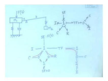
Let us take start with an example that we have already done, the way we did for electrical circuits. For example, this is something that we already did mechanical system with this, this connected to the ground with some force acting on it, this is what we did earlier. A system with a mass spring damper arrangement connected to the ground with a force acting on it and this is a lever with a b ratio and here is another mass M 2, so this is M 1 this M 2.
