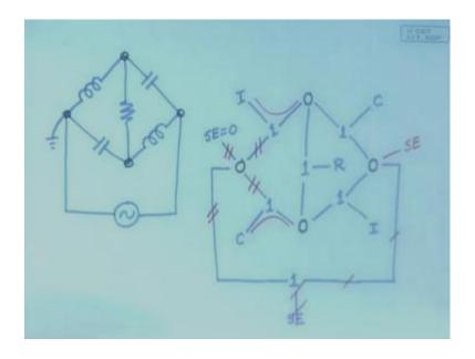
So, this is a source, source of effort. Now, in this case can you see what is connected in series and what is connected in parallel, it is not immediately evident. And in such cases and if such a thing is part of a larger network of elements, it becomes difficult to figure out how to connect this series or parallels. So, in that case it will be convenient to go by that procedure. So, we can identify in this circuit at least a few nodes, this will be a node
