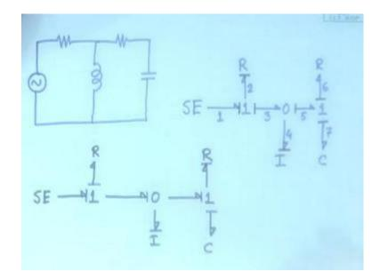
A simple circuit that does not show any sign of being difficult, no difficulty with the circuit, you can easily connect it. Now, let us draw the bond graph of it, S E connected to I connected to R in parallel with I, here it is a series arrangement of R and C. So, give the power directions which would be somewhat simple, now start giving the causalities S E element will give the flow effort information to the rest of the system. So, the causal stroke should be here.
