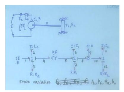
In the motor problem your system description was, you had a DC motor and it was connected to a source, and there would be the internal resistance inductance and this was constant field was constant. This was connected by means of a shaft to some rotational mass, which is allowed to move against a frictional element that was the system description. Now, when we obtained the bond graph how did you go about it, we started from the applied voltage here.
