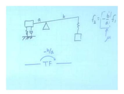
Imagine that you have got something here connected to a lever to something here, so that is also, let it be connected by means of a spring damper arrangement to it is ground, these with a ratio a by b, that also a lever why, because the flow here is related to the flow here by means of what relation, no minus b by a because it goes up it goes down. So, this motion here, so f 2 is minus b by a times f 1, so this minus b by a becomes the mu.
