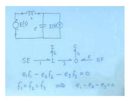
Initially let us start with circuits because they are easier to handle, first it is inductor then we have a capacitor and then we have say a source of flow, this is a E of t, L C this is I of t this is a source of flow. So, it is slightly different, but let us start from one element and then go ahead to draw the bond graph, first let us start with here, so it is a SE element, SE connected to a bond what is it connected to, notice that it shares the same flow with this L element.
