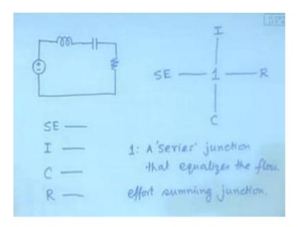
A source of effort connected to an inductor, a capacitor and a resistor, so we know that SE element will be a just like this SE, the inductor will be I, the capacitor will be C and the resistor will be R, but how are they interconnected. Now, that the moment you look at it, you would notice that they are interconnected or they exchange information in a very, very specific way, what is it, that they share the same flow, it is a series connection which means that they share the same flow.
