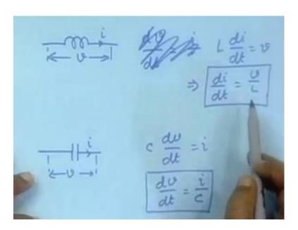
That clue comes from the fact, that if there is an inductor in a specific line and the current flowing through it. Then, we can write the d d v d t as for this L d i d t, so L d i d t is equal to v, so this gives d i d t as v by L, so here is the voltage across the inductor. Similarly, if there is a capacitor in a line, again the current is i and the voltage is say v, then it will be C d v d t is equal to i or d v d t is equal to i by C. So, these are; obviously, differential equations.
