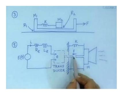
Suppose, there is a cot like think, which is able to move on the ground and this fellow has some mass say M 1 and it is being pulled by a force F. And on this surface, there is a friction, that is say R 1 is consolation, but here is a mass, that is connected by means of a spring, so that is another mass M 2. And here is the K spring constant, I suppose that complete the story, no, there will be some kind of a friction.
