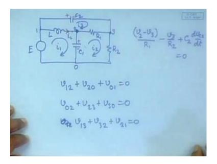
Just let us illustrate it with another example to get it clear, the same example that we have we are doing the 3 loop example, it is a E, then an inductor, then a capacitor, then a resistor, another resistor here and this visible, yes a capacitor, fine. In this case, we will say here is my loop i 1, here is my loop i 2 and here is my loop i 3. So, my E, L, C 1, C 2, R 1, R 2 quickly write the mesh current equations, write the mesh current equations quickly.
