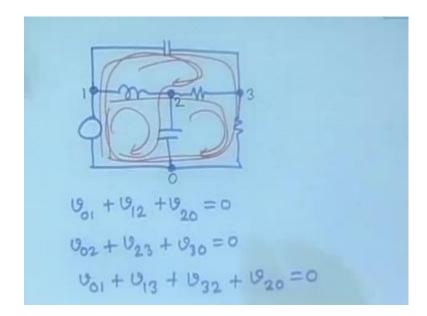
So, suppose you have circuit like this, then what are the loops, well I can identify easily when a loops. This is a loop, all the loops and along around all these, the total voltage should be 0. So, that is the point number 1, that the Kirchhoff's first law. The voltage law says that along, around all the loops the total voltage should be 0.
