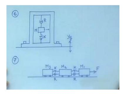
This sixth problem is ever seen a seismograph by which the ground oscillation is measured. So, it is a similar kind of device, say here it is routed to the ground and the whole thing is a hollow box. Inside it, you have a mass spring damper kind of arrangement. So, when this ground moves, this body cannot move instantaneously.
