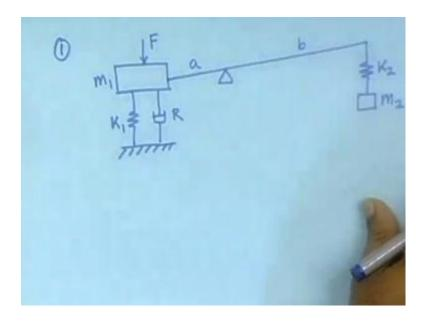
The first problem will consist of a mass, which will be standing on a spring damper support on the ground and if we apply a force that will move up and down depending on the force. But, that is not is the complete story, then is a lever and at the other end of it, there is a mass hanging by a spring. So, there are two masses m 1 and m 2, there is the spring constant k 1 and there is another k 2, there is 1 r and there I have would be also specify the ratio a and b.
