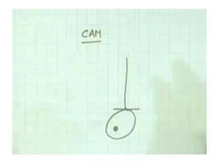
It is something like this, it is called a CAM, where an oval shaped body and there is a plate this is the saft and this is the axis on which it rotates. So, depending on the shape of this, this saft will go up and down, so on this one it is actually forcing a certain flow, you see, it is not giving the force. It is forcing a certain flow, it is a source of flow, it is equivalent to the current source and can you see that, so it is equivalent to current source, it is called a CAM.
