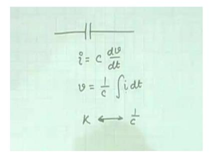
Now, let us talk about the next element, that is the compliant element, compliant element in mechanical was the spring, compliant element in the electrical domain is the capacitance. Here the equation is i is equal to c, that is the equation that we have learnt and where is the slide for the compliant element, spring slide here. Force is k times v d t, here it is the velocity, here the force that is the problem.
