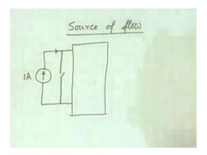
Then, we have to talk about the source of source of flow, in electrical domain; it is the current source, so it is drawn like this, with a certain amount of current, say 1 ampere flowing. There is some kind of system here connected, that immediately says that the current here is dictated by this fellow, a voltage is not. A voltage here, whatever is at work, whatever appears occurs is not dictated by this source elements.
