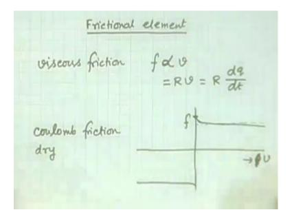
Let us first deal with the viscous friction, for viscous friction the force is equal to or force is proportional, if you can write in this way, force is proportional to the relative velocity between the two bodies. And we will in general, represent that proportionality constant as R, because it is a resistive kind of element, we will in general denote it as R. So, this equal to R, so the relative change in the position in terms of that, if you write it is d q d t.
