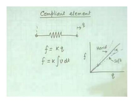
The second element that we will be considering is the compliant element; the compliant element is essentially the spring. So, these two extremities have certain positions in the unstaged condition and if you pull it, thereby change the position. Suppose, these two position, suppose this is fixed and this is defined by the position variable q and you are pulling it, what happens, what is the terminal characteristic, I am not concerned about, what happens inside the spring.
