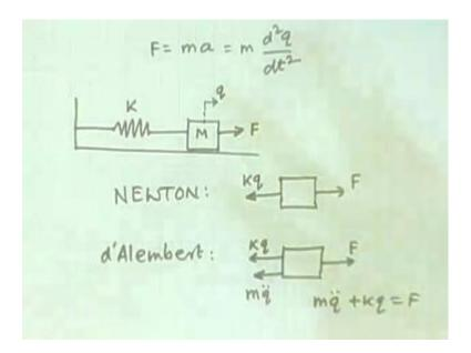
So, let us start what we will do is, first let us go by the mechanical way; that means, let see the mechanical systems and in the mechanical systems, you know the elementary equation is given by Newton. That is force is equal to mass into acceleration or this being a double derivative of the time, immediately you can seen that this is the differential equation, so simple. For anything, if you can identify the force, you can identify the mass; then you can write down the equation.
