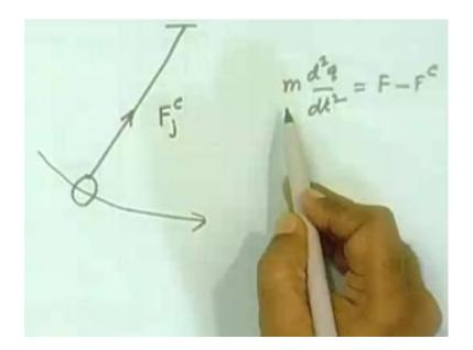
If you have a pendulum, now what is the constraint, now in that case pendulum moves like this it is constraint to move on the surface of a sphere, it is constant to move on the surface of a sphere, this fellow is constant to move on a plane. If you have a planar pendulum; it is constraint to move on a circle. So, these are constraints and have you ever ridden on a roller coaster in the phase, you are made to move in a specific strategies stomach turning thing.
