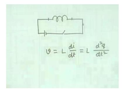
Notice, that if you consider, suppose we consider a inductor and you have got some kind of voltage source and switch what is the character of this inductor as seen between the terminals. It is some kind of a relationship between the voltage and the current and what is the current, what is the relation, simply stop. Now, the current is the rate of change of rate of flow of charge.
