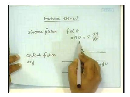
So, that is the property of the resistive element, but you notice that the resistive element in general is exactly the same as the viscous friction element in the mechanical domain. Because, here the force is R times the velocity, here the force is R times capacity clear, so we have established the equivalence of the electrical and mechanical system.
