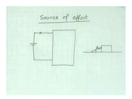
There are two other elements that would require a various tension, one is the voltage source and we will in general name it as source of effort. In electrical domain, that is the voltage source, in a mechanical domain has the external applied force is something is
