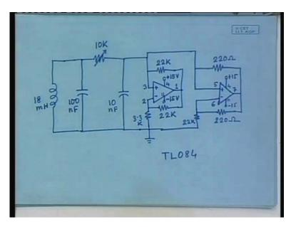
Here you have the inductor, if you want to make it you will made this complete circuit diagram. This is 18 milli Henry. Here there is a capacitor, it is 100 Nano Farad. There is a resistance which is 10 k, easily available component there is no difficult in making it, this fellow is 10 Nano Farad. Now comes the the non linear element that will have this property. It is actually realized by 2 op amps, op amp 1 and op amp 2.
