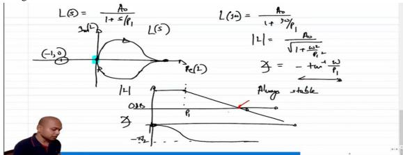
So, the magnitude of the loop can goes to 1 where the loop can crosses the 0 dB line and that frequency at which it crosses is called unity gain frequency right or omega U G B right.
