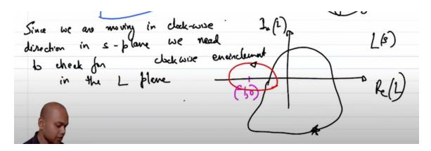
So, this is stable right this is still stable ok. So, we have to keep a track of whether the encirclement is a clockwise or anti-clockwise direction ok.
