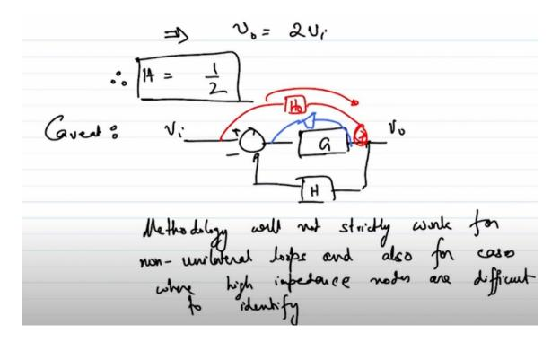
So in that case this methodology will strictly not work but a modified version of this method methodology is going to work right. So in this course we'll not get into that we don't have the time and the bandwidth to get into those details. But the circuit that we'll be dealing with in this course will have places to break where this where the simplistic GH kind of methodology will still work. So we will stick to that right. Thank you.
