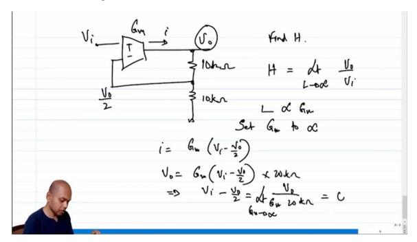
So in other words Vi minus V0 over 2 is equal to V0 by gm times 20 kilo ohm. Now limiting value of this guy when gm tends to infinity is what? This is 0. Which means what? Which means V0 is equal to twice Vi correct. So which means what is h? Oh I made a mistake sorry.
