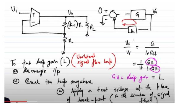
another if things go in other if you have multiple loops or you have multiple current directions then things can be can be slightly different ok. So, we should keep that in mind, but for the purpose of this course this is good enough. Then what should we do? Then we should apply a test voltage here in the direction of signal flow let us say Vtest right.
