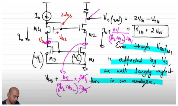
Since the drain voltage of M2 is not the same as drain voltage of M4 the incremental current right. So, that the current in both the branches will also not be identical to the nth
