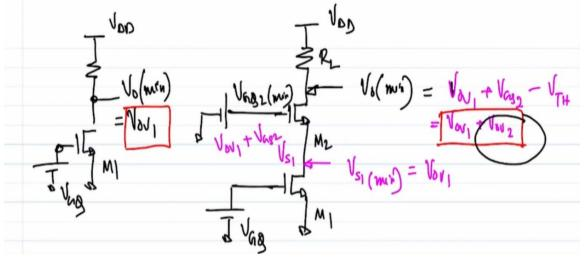
So, you see that in the circuit on the left the minimum output voltage is 1 over drive voltage of M1 in the circuit on the right the minimum over drive minimum output voltage is the
