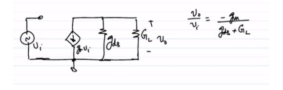
So, what was the solution? The solution that we came up with was use a current buffer, right. So, what is the current buffer? Again, a current buffer is a contraption that helps in pushing the current from a non-ideal current source to a load without the effect of loading, right. So in our case, our ideally, in our case, so this non-ideal current source was this section of GM, Vi and GDS, right.
