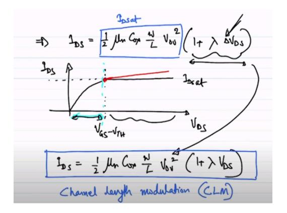
So, now what impact will this have on our incremental characteristics? Clearly you see that the Y 2 2 for this characteristics will not be 0 right. So, that will be a significant that will have a significant impact on our current voltage characteristics of the device, but
