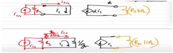
So, if this is I1 this is I1 and the output is flowing into Rd parallel Rl right. So, this essentially is what is happening in the incremental feature in the circuit on the top. So, now, we while we ended the previous lecture I had requested you to find out if Iin is a sinusoidal waveform right if Iin is equal to Ip sin omega naught t. So, let us see say if Iin is equal to Ip sin omega naught t what will be the constraint on Ip correct. So, what I
