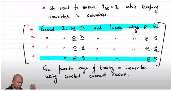
So how many possible combinations of applying the current source and tweaking the gate and source voltage can I come up with? Clearly, I can come up with four possible combinations, right? So the first combination was connect I0 at drain and tweak voltage at gate. This is what we did in the previous lecture. What are the other options? Obviously, the other one of the other options is connect I0 at drain and tweak voltage at source, right?
