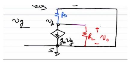
The transistor is a gm a voltage control current source the source is grounded right source is grounded. So, we do not have to bother too much on top I have Rd right. What is what should I do with the other side of the Rd? Other side of the Rd should be grounded because again Vdd right.
