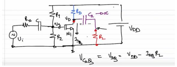
So, what is this voltage? That voltage is 0 what is Vd? Vd is Vdq right. So, Vc2q is Vdq which is Vdd minus Idq rel right. So, the so note that by putting a capacitor we are not disturbing the we are not disturbing the quiescent point of the other transistor right. If we can ensure that we are not disturbing the quiescent point of the transistor that is a good start
