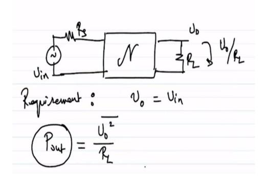
So, that that essentially is one of the main motivations of this course as to how do I design this network N which can give me the required amount of power regardless of whatever the load might be so that I am able to hold certain voltage across it or if the application requires I am able to supply certain current through it ok?
