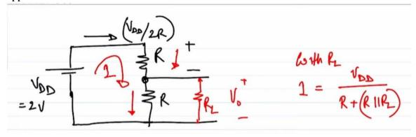
In other words what we are asking what we are asking is how can we mitigate how can we reduce the extra drop across R once we connected RL right. So, in other words what we are asking is how can we reduce the extra drop across R when RL is connected? So, this is the question that we are asking. So, in order to answer this question we need to figure out which value of RL causes the most problem.
