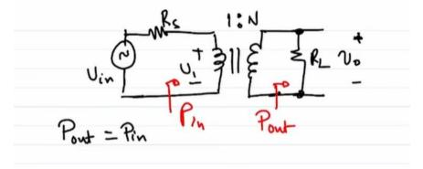
So, whatever power goes in inside the transformer none of it can get dissipated in the transformer and the transformer cannot generate any power on its own which means the power that is going into the transformer only has one place to go and that is into the load resistance which gets dissipated, but which consumes the entire power that went inside the transformer.
