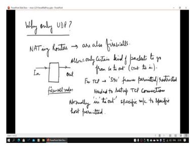
So why use only UDP? NATing routers normally are also firewalls and they allow only certain kind of packets to go through from in to out or from out to in. These are going to be firewall rules. So, we use IP tables, for example in any Linux machine for doing this job. For TCP frames normally there is a sync frame which is transmitted. So, when IP packet comes in, we actually look into the payload these firewalls look into the payload, whether it is a TCP
