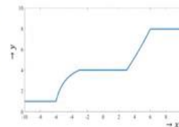
Overall Input Output Curve for Single-Input Single-Output Mamdani Fuzzy Model
