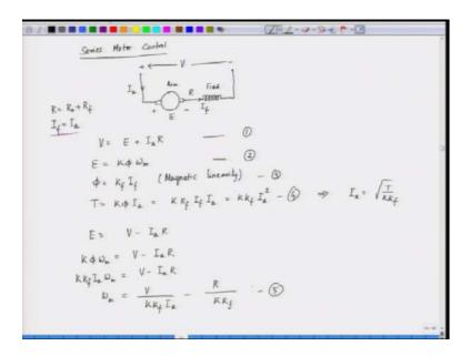
The back EMF E appears across the armature, and the voltage equation for the series motor can be written as:
