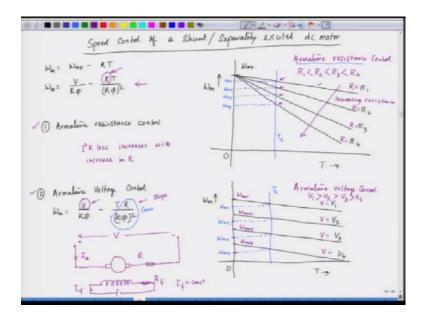
This is the speed-torque characteristic of a separately excited DC motor. The speed, denoted by  $\omega_m$ , is given by the equation:
