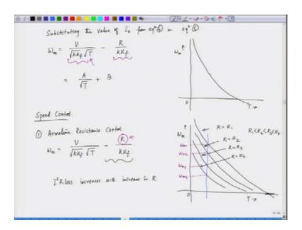
By substituting the value of  $I_a$  from equation (4) into equation (5), we get the expression for motor speed  $\omega_m$  as:
