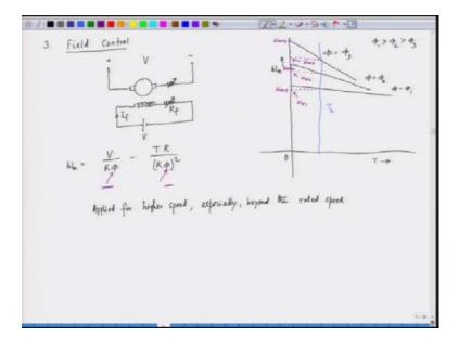
The third method of speed control is through field control, also known as field current control. In this approach, we focus on controlling the field current, which directly influences the magnetic flux  $\phi$  of the motor. Imagine we have a separately excited motor with the armature connected to a voltage source V, and the field winding with resistance  $R_f$  also connected to the same voltage source.
