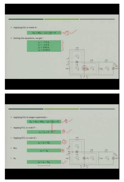
We will write KVL for this mesh, so what we can write?  $2i_4 + 8(i_4 - i_3) + 10 = 0$ , so, you will get another equation here. Now, what you have to do? You have to utilize this, this, this and anywhere we have utilized this and put the value inside the equation 3 and we get  $i_2 = i_3-3i_4$ .
