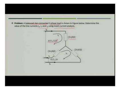
Now, another example which you can take and this is very common example you will see in book, this is balanced star connected 3-phase load and we need to determine the value of currents flowing through R, Y and B phase. So, here also we can apply the mesh current analysis, the voltage a line to line voltage that is voltage across R and Y is given as  $415 \ge 120$  and between Y and B is  $415 \ge 0$  and this is balanced 3-phase load, so the impedance is across the loads is 3 + j4.
