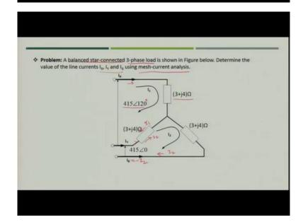
Now, you have both of the equations available you have to just solve these two equations and you will get the values for current I 1 and I 2. Now, line current which you will see in this figure,  $I_R = I_1$ ,  $I_Y = I_2 - I_1$  and  $I_B = -I_2$ .
