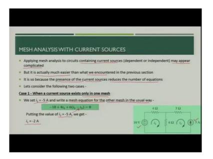
Now, that particular case was relatively simple because mesh the current source was in only one mesh. But suppose if the current source exists between two meshes where the both of the meshes are sharing the current source then what you have to do? You have to analyze the circuit by creating a super mesh, super mesh means? You have to exclude the current source and any element connected in series with that particular source.
