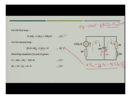
If you rearrange and solve this equation the current  $I_1=10.77 \angle 19.23^{\circ}$  A =  $10.8 \angle -19.2^{\circ}$ A and  $I_2=10.5 \angle -56.7^{\circ}$ . Now, here you can see that the result would come in the form of rectangular coordinate where you will have real component as well as imaginary component. So, using your previous knowledge of phasor calculation you can find out the value of these currents in terms of phasor also.
