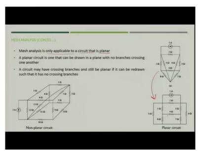
Yesterday we also discussed that the mesh analysis is only applicable to circuit that is planar, planar means the circuit which can be drawn on a plane and it does not have any branch which are crossing one another. So, like in this case if you see it is not a planar circuit because it is not drawn on a plane it is something like three-dimensional structure. Similarly, here also we saw that it is crossing the branches but we can reorganize and make it as a planar circuit.
