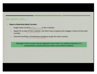
And we saw that the three steps are required for the mesh analysis we have you will first define the mesh currents then you apply KVL at each of the n mesh and then solve the n simultaneous equations.
