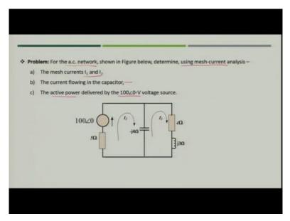
Now, let us talk about another example. Now, this example is not the dc network it is related to ac network as shown in the figure below and now the objective is to determine the mesh current I 1 and I 2 and the current flowing in the capacitor and active power delivered by 100 voltage with reference phasor as 0. So, we will use this circuit and try to apply the mesh analysis technique and find out the result.
