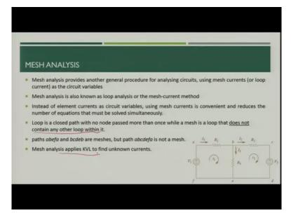
So, yesterday we saw the what is mesh analysis and we stabilized the difference between the mesh current and the branch current and we also saw that every loop cannot be considered as mesh because mesh is that loop which does not contain any other loop within it and we also saw that the mesh analysis can be done with the help of Kirchhoff Voltage Law.
