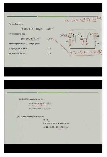
Now, next the source power that is basically the active power you need to calculate. So, active power is  $P = VI \cos \varphi$ , here voltage V is a difference phasor because it is generally 0 so we are considering it as a reference phasor and then you have to simply put the value of current, current would be what? Current is flowing from the source, so what is the current? Current would be essentially the value of  $I_1$  because this is the current which is flowing from this particular site.
