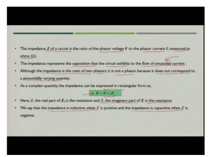
The impedance of a circuit is the ratio of voltage phasor and current phasor and it is also measured in ohms. Because in case of resistor or capacitor or inductor, whatever the reactance is which we calculated in previous lectures. The dimension of those was in ohms. Now impedance represents the opposition that circuit exhibits to the flow of sinusoidal current.
