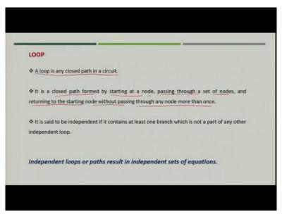
Now what is loop? In any closed path loop is basically a closed path in any circuit. The closed path formed by starting at a node, passing through a set of nodes and finally returning to the starting node without passing through any node more than once.
