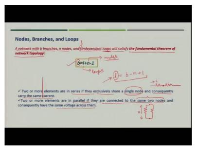
Now the question would be, how you will find out whether you have got the correct number of loops or not? For that we use the fundamental theorem of network. So, b=l+n-1, l is the number of loops, n is number of nodes and b is number of branches. So, you know you can find out the numbers of nodes, you can find out the number of branches, so you can easily find out what would be the numbers of loops, so l would be nothing but b minus n plus one.
