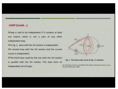
So that means if you see the circuit like this when you are ask to find out the loop, it means that if you trace out various nodes and come back to the original node then this will consider to be one loop, right.
