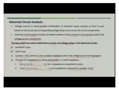
We will try to analysis the circuit and try to find out the currents which are there in the various branches of the network and the voltage across the components. Let us recap what we discussed till now related to circuit analysis. There are various laws which are used to determine the currents and voltage drops in the electrical circuit. We discussed about the Kirchhoff's law, we also discussed Ohm's law, Ohm's law is nothing but the finding out current I = V/Z.
