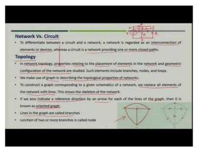
Now let us talk about the network. Till now we have discussed like every time we use electrical circuit not the network. So, what are the difference between network and circuit? The difference between a network and circuit is that the network is an interconnection of elements or devices. That means that it is not necessary that it will create a close loop, so it can have the close loops but there may be some open loops also.
