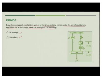
Now, let us try to understand what we have just now discussed with the help of one example. So, in this example we need to draw the equivalent mechanical system of the given circuit, given mechanical system. Now, write the equilibrium equations for it and obtain the electrical analogous circuit using force voltage and force current analogy.
