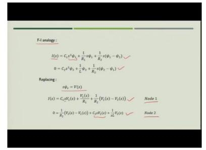
Which is basically can be represented with the help of this particular circuit. So, if you see here you have the C1 and R1 these are in parallel. So, C1 R1 in parallel then you have current source I1 which is now connected to V1, between V1 and V2 you have the resistance that is 1 /R2.
