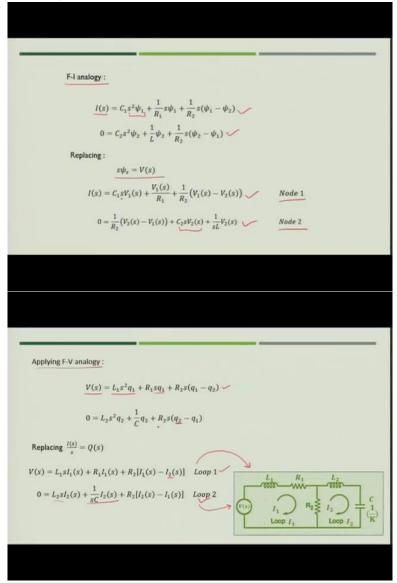
Now, the second case is that you can create the force current analogy also. So, in that case what you can do? You can instead of writing the equation for voltage analogous we will write the equation for current analogous. Then we can write,
