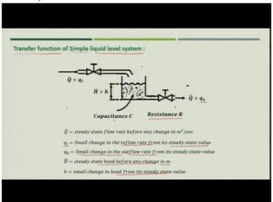
Now, let us see the transfer function development for say simple liquid level system where you have some steady state flow Q which is going inside the tank, the water is flowing and suppose there is a small change in the inflow rate from its steady state value which will cause the small change in the head from a steady state value. So, when you change the inflow rate the head will increase.
