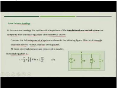
So, first we will see what is the force current analogy? So, the force current analogy the mathematical equation of the translation mechanical system are compared with the nodal equations of the electrical system. Now, consider the following electrical system which is shown in the figure. Now, this circuit consist of current source, resistor inductor and capacitor. So, all are connected in parallel.
