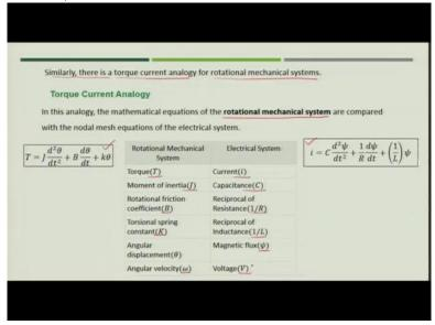
Now, the same concept we can utilize for torque current analogy also that is basically applicable for rotational mechanical system. When we apply torque current analogy then the mathematical equation for rotational mechanical system we get
