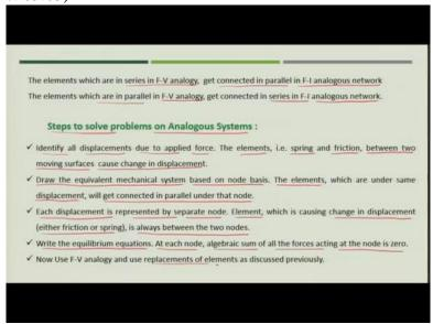
Now, the elements which are in series with force voltage analogy get connected in parallel in force current analogous network. Similarly, the elements which are parallel in force voltage analogy get connected in series in force current analogous system. Now, let us try to understand how to solve the problem on analogous systems. So, what are the various steps that we can follow to solve the problem?
