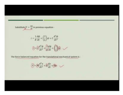
We will get the analogous quantities of the translational mechanical system and the electrical system. So, if you see these two equations you can say that force and current has the analogy M that is mass is analogous to C, B is analogous to 1/R, K is analogous to 1/L, x is analogous to  $\psi$  and you can also say dx/dt that is velocity v is analogous to  $\frac{d\psi}{dt}$  that is nothing but voltage V.
