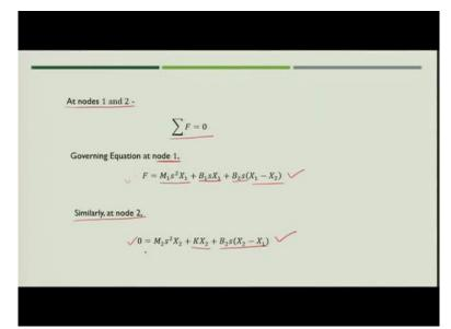
Now, if you use force voltage analogy, you can simply write these two equations in the corresponding analogous voltage equations. So, what we can write, we can write,
