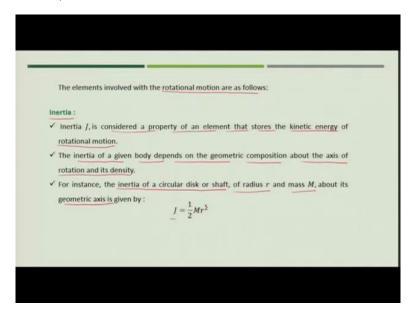
Now, the elements involved in the rotational motions are first inertia. So, inertia is considered as the property of an element that stores the kinetic energy of the rotational motion. So, you can correlate it with respect to the mass m which we discussed in case of translational motions. So, here also the inertia is the property of element which stores the kinetic energy of rotational motion.
