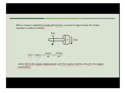
Now, when the torque is applied to a body with inertia J, if you see the figure, the body which is rotating having inertia J and it is having  $\theta$  as the displacement and when the torque is applied, the governing equation which you can write is
