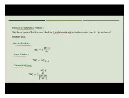
Now, similar to what we saw in case of translational motion, in this case also we will see various frictions. What are those frictions? First is viscous friction that is torque  $T(t) = B \frac{d\theta(t)}{dt}$ . This B is called a viscous friction coefficient. Then static friction, in that case the friction torque  $T(t) = \pm F(s)|_{\dot{\theta}=0}$  that is the object is just about to move.
