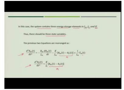
Now, let us assume that we have 3 state variables  $x_1(t) = \theta_m(t) - \theta_L(t)$ ,  $x_2(t) = \frac{d\theta_L(t)}{dt}$ , and  $x_3(t) = \frac{d\theta_m(t)}{dt}$ . So, the state equations which you can write, if you differentiate,
