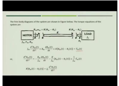
Now, in this case the system contains 3 energy storage elements that is  $J_m$ ,  $J_L$  and K. So, what we will do, we will find 3 state variables in this case. The equations which we just saw in case of the motor side and the load side free body diagram, we came with these 2 equations that is
