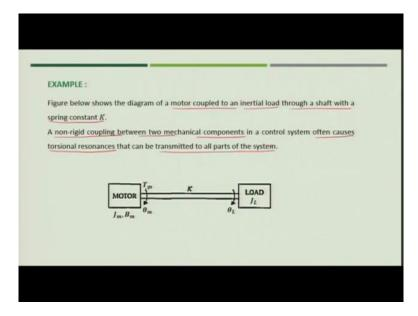
Now, let us take one example so that we can understand how we will create the mathematical model of mechanical system. So, in this mechanical system we have one motor connected to a load through shaft which has the friction coefficient as we will rather say stiffness coefficient as K which defines the torsional spring coefficient. Now,  $T_m$  is the mechanical torque applied by the motor and  $\theta_L$  is the displacement at any time t for the load which is having inertia equal to  $J_L$ .
