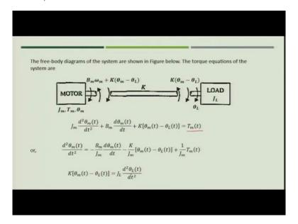
So, from the motor side, if you see the free body diagram you will see that the torque  $T_m$  when it is applied, you will have the viscous friction part plus spring torque part applicable in the opposite direction of the motor torque applied. The torque equations of the system are
