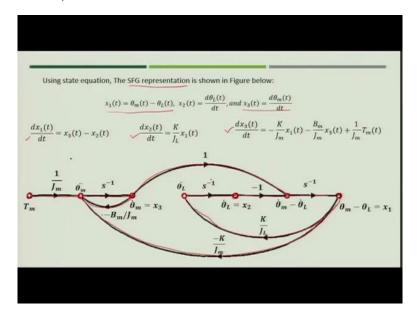
We can represent the state equations which we have just got using the signal flow graph. So, how we will represent? We have defined the state variables as  $x_1(t) = \theta_m(t) - \theta_L(t)$ ,  $x_2(t) = \frac{d\theta_L(t)}{dt}$ , and  $x_3(t) = \frac{d\theta_m(t)}{dt}$ .
