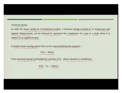
Now, like the spring, linear spring which we saw in case of translational motion, we can also define torsional spring. Torsional spring let us say we have a torsional spring constant K that is given in torque per unit angular displacement, so we can devised to represent the compliance of a rod or a shaft when it is subject to applied torque. So, torsional spring is the property of the shaft or the rod which is connected to your rotating body.
