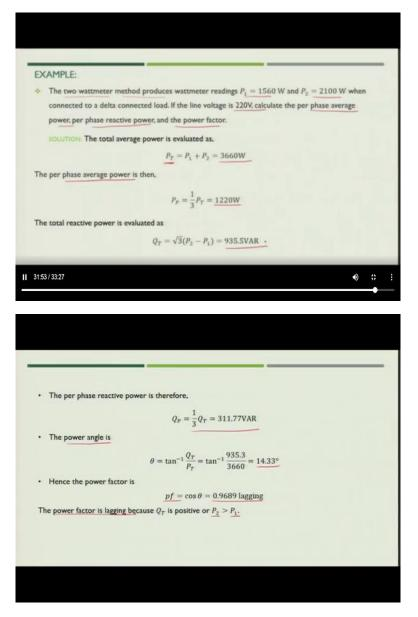
Now, let us see quickly the third method also, third example also where we need to use the two watt meter method to find the value of per phase average power, per phase reactive power and the power factor  $P_1 = 1560$  W and  $P_2 = 2100$  W is given and the line voltages is 220 volt. Since P 1 and P 2 is given total power average power you will get as
