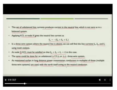
Now this set of unbalanced line current produce current in the neutral wire because the total sum of line currents, that is  $I_a + I_b + I_c$  will not be 0 which we saw in case of balance system. So in that case if we apply KCL at node N we get the value of neutral current that is
