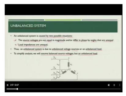
Balanced source is behind the particular nodes, which we are seeing so we are not showing that in the figure but since our objective is to analyze the circuit by assuming unbalanced load.
