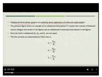
So in that case for the unbalanced three phase system, the various electrical parameters can be calculated by direct application of either mess of nodal analysis. So in the figure which we just saw in this slide this is an example of unbalanced three phase star star or you can also say Y Y system that consists of balance source.
