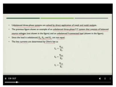
We are showing only the unbalanced load in the figure. So, we will see only the unbalanced load as we saw in the previous figure. Here in case of unbalanced load  $\mathbf{Z}_A$ ,  $\mathbf{Z}_B$ , and  $\mathbf{Z}_C$  are the phase impedances which are not equal. Now when we calculate the line current, we calculate the line current with the help of Ohm's law.
