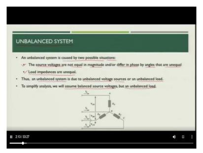
Let us start our discussion of today's lecture. First let us understand what unbalanced system is. So, unbalanced system is caused by two possible situations. What is that? The source voltage is not equal in magnitude and or differ in phase by angle that are unequal. That means for a balanced system we generally know that the phases are equally upon equally distant with respect to each other that is 120 degree apart from each other.
