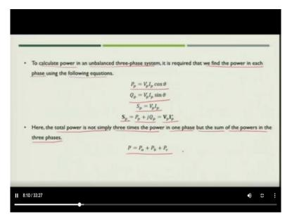
Now to calculate the power in an unbalanced three phase system, what we require? We require that we find the power in each phase using the equation which we have seen earlier also. So like real power in phase we can write as,
