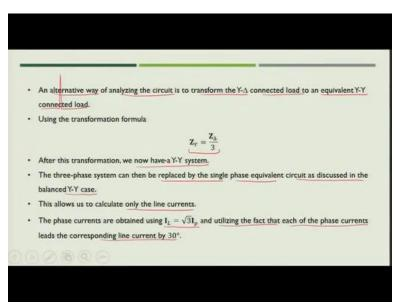
Now there is an alternate way also to analyze the circuit to transform star delta connected load to equivalent star star connection. In that case what you have to do, you have to convert delta connected load into equivalent star connected load which we can do with the help of star delta transformation. In that case you can say  $\mathbf{Z}_Y = \frac{\mathbf{Z}_{\Delta}}{3}$  and when you put you can analyze the system as we did in case of star star connection.
