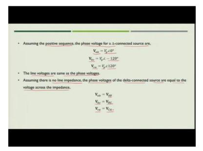
Now if we assume positive sequence that is the sequence is A, B, C the phase voltage for a delta connected source will be,
