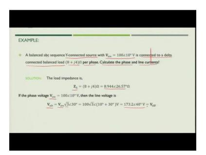
Now let us take 1 example. Suppose there is A, B, C phase sequence star connected source with the phase voltage  $V_{an} = 100 \ge 10^{\circ}$  V and it is connected to a delta connected balanced load with impedance  $(8 + j4)\Omega$  per phase. We need to calculate the phase and line currents. So, the load impedance you can convert it into phasor form as,
