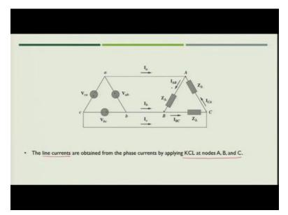
So now you have the phase current information. Next task is you need to find out the line current. So how you can find out the line current, you can simply apply KCL at the nodes either A or B or C you can apply the KCL. So here if you apply the KCL, you will get
