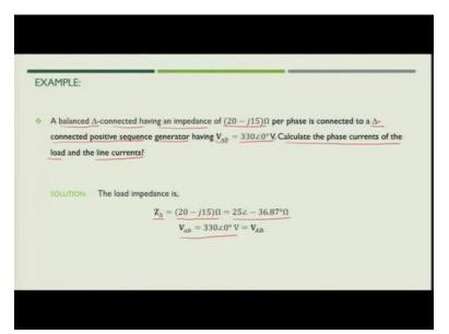
Now let us take the example related to our balanced delta-delta connection. In this case the balanced delta connected load having an impedance of  $(20 - j15)\Omega$  is connected to a delta connected positive sequence generator having  $V_{ab} = 330 \angle 0^\circ$  V. What we must find out, we have to find out the phase current of the load and the line currents of the circuit. We can convert it into phasor as,
