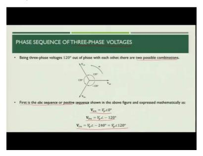
When we talk about the three-phase voltage source phase sequence we see there are two possible combination of phase sequencing.
