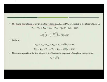
Now if you are asked to find line to line voltage or simply the line voltage, line voltage would be  $\mathbf{V}_{ab}$ ,  $\mathbf{V}_{bc}$  or  $\mathbf{V}_{ca}$ .
