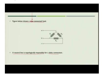
Now next combination is delta connected, so this is basically the delta connected configuration. Here you will see *abc* are connected in triangular fashion and your phase ABC is taken out from the load and if you see this arrangement in this particular arrangement you cannot take the neutral connection out because it is topologically impossible to take the neutral connection from the delta connected load.
