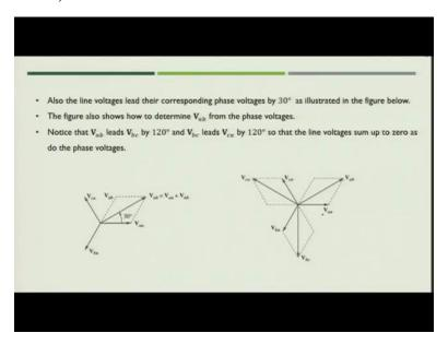
So, in the line voltage you will see that these are leading with respect to their phase voltages by 30 degree, so we also see that the line voltage is now root 3 times of the phase voltage in magnitude.
