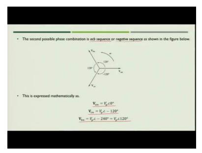
Now next possible combination is *acb* sequence which is called as a negative sequence, so in that case what happens that you are reference phasor that is  $\mathbf{V}_{an}$  leads  $\mathbf{V}_{cn}$  and  $\mathbf{V}_{cn}$  leads  $\mathbf{V}_{bn}$  by 120 degree, so what we write mathematically,
