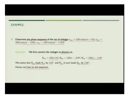
Now let us take one example in which we need to determine the phase sequence of the set of voltages like  $v_{an}=200\cos(\omega t+10)$ ,  $v_{bn}=200\cos(\omega t-230)$ ,  $v_{cn}=200\cos(\omega t-110)$ . What we have to do first, first we will convert it into phasors, so  $\mathbf{V}_{an}=200\angle10^\circ$ ,  $\mathbf{V}_{bn}=200\angle-230^\circ$ ,  $\mathbf{V}_{cn}=200\angle-110^\circ$
