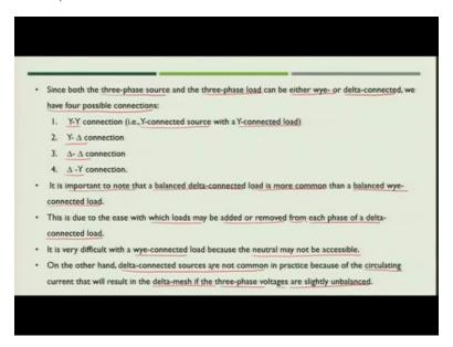
Now since you can have source and load both three phase connected in either star or delta connected fashion, so we can have now four possible combinations of the connections between source and load as.
