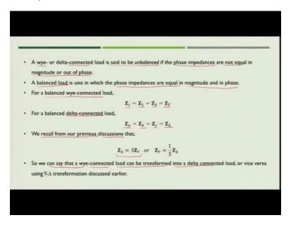
Now whether it is star connected or delta connected will say that if it is unbalanced then the phase impedance will not be equal, and the phase sequence will also be out of phase.
