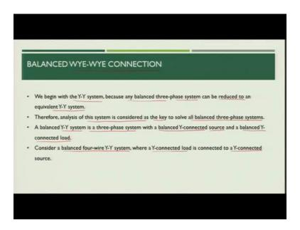
Now let us talk about the connections we saw that there are first four possible combinations that is Y-Y, Y delta, delta-delta and delta-Y connections between source and load, so we will first start with Y-Y connection for the source and load, why we are starting with Y-Y connection because any balanced three phase system can be reduced to a Y-Y system with the help of star delta transformation, so therefore this system is considered as a key to solve the all balance three phase system.
