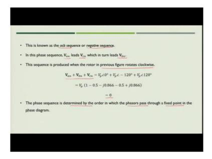
So, here now the sequences acb sequence all you generally call it as a negative sequence. So, in this case  $\mathbf{V}_{an}$  leaves  $\mathbf{V}_{cn}$  and  $\mathbf{V}_{cn}$  leads  $\mathbf{V}_{bn}$  by 120 degree. Now, so, sequence is produced when rotor is rotate in the rotor is rotating in the clockwise direction. So, here now, if you calculate,
