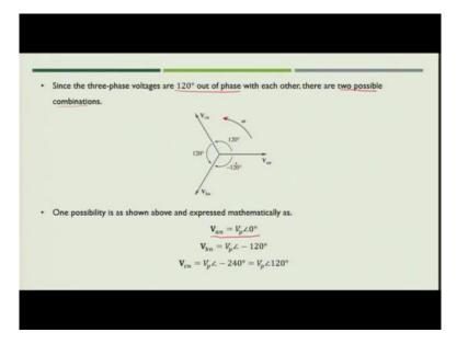
Here V<sub>p</sub> is the effective or RMS value of the phase voltage.
