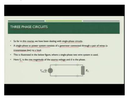
Now, let us start another topic, which is 3 phase circuit. So, till now what we have discussed in our course was basically related to single phase circuits. So, in case of single phase the power system we consist of 1 generator connected through a pair of wires or we call it as transmission
