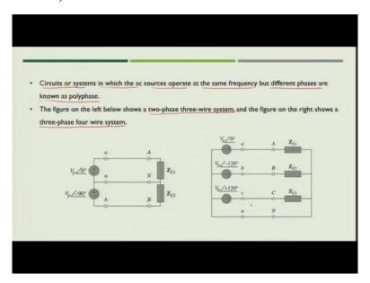
Now, there are circuits or systems in which ac source operate at the same frequency, but there may be different phases So, we call them as poly phase circuit. So, if you see the figure below, you will see on the left there are 2 voltage sources connected to the load with the help of 3 transmission lines and load  $Z_{L1}$  and  $Z_{L2}$  are connected. So, if you see these 2 sources, 1 is  $V_p \angle 0$  another is  $V_p \angle -90$ .
