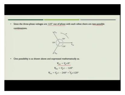
So, now, since the voltages are 120 degree out of phase, there are 2 possible combinations for the arrangement of these phases. So in 1 such arrangement is shown in this slide, where  $\mathbf{V}_{an}$  is leading  $\mathbf{V}_{bn}$  by 120 degree and  $\mathbf{V}_{bn}$  is again leading  $\mathbf{V}_{cn}$  and by 120 degree. So, what you can write,
