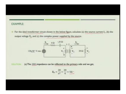
Now, suppose if the ideal transformer contains the circuit as shown in the figure below, we need to calculate the source current  $I_1$  and the output voltage  $V_0$  and complex power supplied by the source. So, in this case, you will see that the 20 ohm is the load impedance. So, to simplify what we first have to convert that load impedance in such a way that it is reflected to the primary side.
