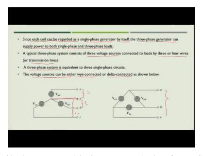
Now, let us consider the star connected that is wye connected voltage for now. So, here we will have phase voltages as  $V_{an}$ ,  $V_{bn}$ , and  $V_{cn}$ . So, these are respectively the voltages between line abc and the neutral. So, we have seen that  $\mathbf{V}_{an}$  is nothing but what is between a and n and lines  $\mathbf{V}_{bn}$  is between b and b are called phase voltages because you have taken them with respect to neutral.
