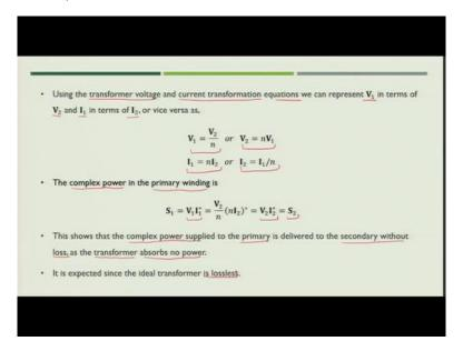
Now, let us see other aspects of the transformer using transformer voltage and current transformation equations, we can now represent voltage that is primary site voltage in terms of secondary site voltage and primary current in terms of secondary current or vice versa. So, what we can say, we can say
