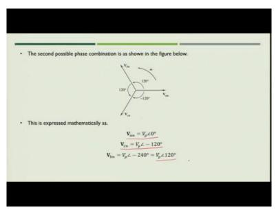
Now, there is another phase combination where  $V_{an}$  leads  $V_{cn}$  which in turn leads  $V_{bn}$ . So, in that case what you can write, you can write,
