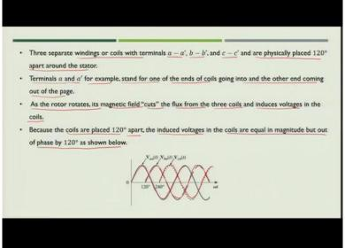
Now, these separate winding or coils which you see as a - a', b - b', and c - c' in the figure. Basically, we arranged the coils in such a way that it completes 1 set of arrangement for 1 particular phase. They are physically 120 degree apart around the stator. So, if you see A and B, so, the angle difference will be physically 120 degree. Similarly, between B and C and between A and C will be also 120 degree.
