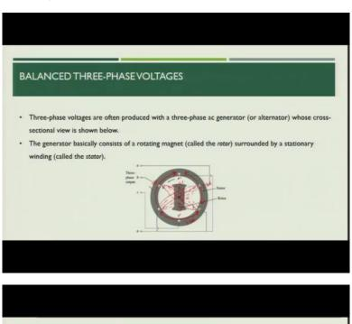
Since each coil can be regarded as a single-phase generator by itself, the three-phase generator can supply power to both single-phase and three-phase loads.
