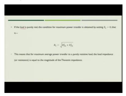
Now, in case of ac if your load is purely real what would be the condition? The condition for maximum power transfer will be obtained by setting XL is equal to 0.
