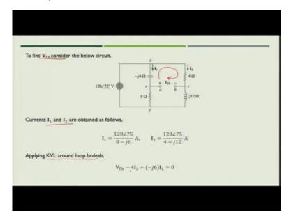
Next task is, to find out the Thevenin voltage. So Thevenin voltage is nothing but the voltage across the terminal a b. So, how to solve, we will first try to find out the currents I1 and I2. I1 is flowing in the d f segment and I2 is flowing in the right side of the segment. So
