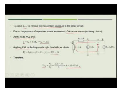
If you remove the current source the updated circuit will be like shown in the figure and now, across terminal a b we apply a current source having value 3 ampere. We have taken 3 ampere as an arbitrary choice you can assume any value. The Thevenin impedance  $\mathbf{Z}_{Th} = \frac{\mathbf{v}_s}{\mathbf{I}_s}$ . If you apply KCL at the node,
