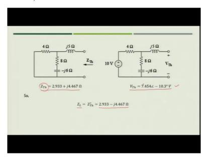
So, you will get the circuit like this. To find out the Thevenin impedance you will short circuit this. So your circuit will become like this. And this 4 ohm resistance will now be in parallel with 8 ohm resistance in series with minus j 6 ohm reactant. So, if you solve this, the parallel combination of this and then the result is added with j 5 ohm reactance offered by the inductance you will get Zth as 2.933 plus j 4.467 ohm.
