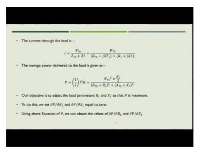
Now, next is you need to find out the current which is flowing through the load. So what is the value of current? Current is nothing but Vth divided by the Zth plus ZL. So, that is Zth plus ZL. Now, you simply replace the values with the rectangular form of the Zth and ZL.
