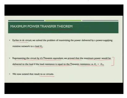
Now, let us come to the, another theorem called Maximum power transfer theorem. So, in case of dc circuit we solve the problem of maximizing the power delivered by the power supplying network to load RL. So, how we solve? We solved mathematically and saw that the first the circuit is represented by its Thevenin equivalent and then mathematically we prove that maximum power would be deliver to the load, if load resistance is equal to Thevenin resistance.
