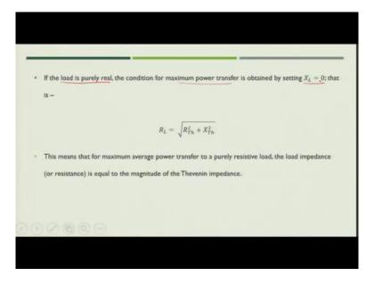
So, in case of dc, the maximum power transfer was obtained by setting RL is equal to Rth, but in case of ac the value of RL would be equal to under root of Rth square plus Xth square. So, what does it mean? That means that the maximum power transfer to a purely resistive load the load impedance that is the resistance in this case will be equal to magnitude of the Thevenin impedance.
