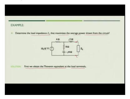
Wwhere you have 10 volt, 4 ohm,8 ohm and minus j 6 and j 5 ohm connected.
