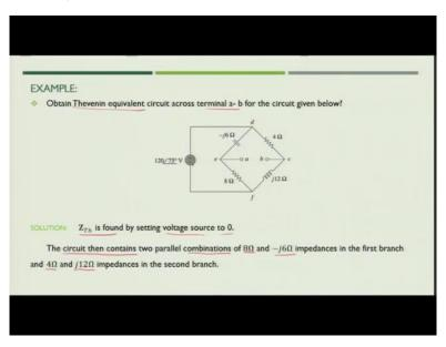
So, if you go back to the circuit f and d are not short circuited because you have put voltage source as a short circuit.
