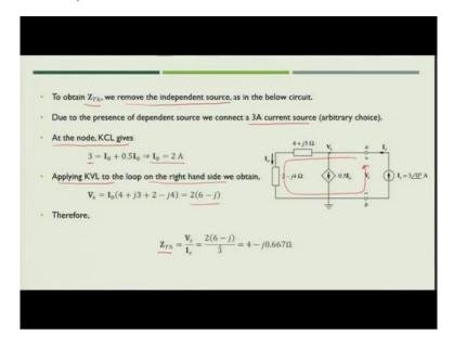
Next task is you need to find Zth. So, to find the Zth we remove the independent source. So, independent source in this case is the current source.
