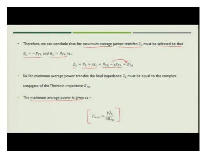
So, this is what you get under the maximum power transfer condition. So, if you compare from the dc circuit this is slightly different because of the introduction of reactive component in the impedance.
