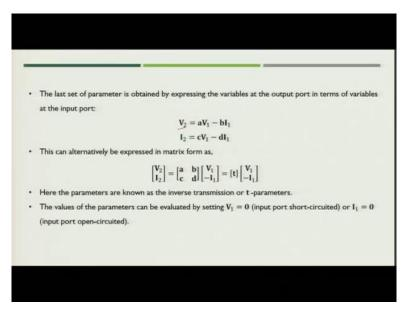
Now, next is the opposite of what we discussed till now means the relationship will now be  $V_2$ ,  $I_2$  will be related with respect to  $V_1$ ,  $I_1$  that means we can also set  $V_1$ ,  $I_1$  as independent variables and  $V_2$ ,  $I_2$  as dependent variables, in that case the relationship which we get is called as a inverse transmission or inverse T parameters.
