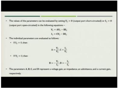
Now, let us see how we will calculate these parameters. The parameters we can calculate by setting  $V_2 = 0$  that means you set the output port as short-circuited or  $I_2 = 0$  that means you set output port open circuit. Now, the equations which we saw in terms of ABCD parameters which relates  $V_1$ ,  $I_1$  and  $V_2$ ,  $I_2$  is like this shown in the slide,
