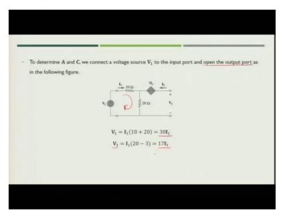
So now, in first case what we are doing? We are opening the output port and the input port we have a voltage connected that is  $V_1$ . And when we have this particular condition, we put these values in the ABCD equation that is  $V_1$ ,  $I_1$  equations.
