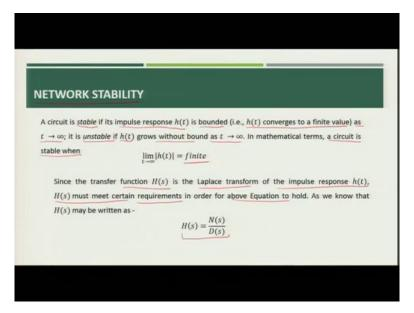
Now let us move on to another concept called network stability, here the circuit is stable if its impulse response is bounded, means the h(t) converges to the finite value when  $t \to \infty$  and if it is unstable if s t grows without bounds s  $t \to \infty$ . So, in mathematical terms you can say that the circuit is stable when,
