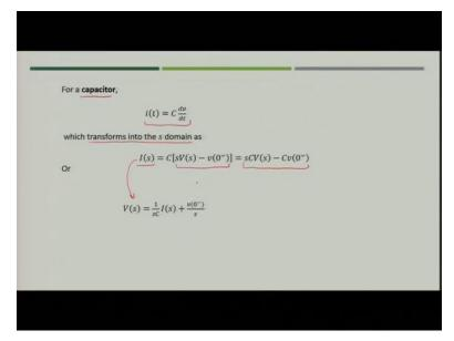
Now, next let us talk about the capacitor so, in case of capacitor we know current at any time t can be given by  $i(t) = C \frac{dv}{dt}$ . So, using the equation in time domain we will transform this into s domain. When we convert it into s domain it will become
