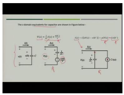
So, let us see how we will represent the equivalents of capacitor in s domain. So, this is the (equal) equivalent representation of capacitor in time domain where you have voltage across capacitor as v(t), initial voltage across capacitor is v(0).
