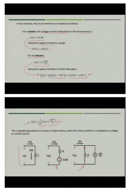
Let us first see the three key elements which we generally have in our circuit those are resisters, inductors and capacitors. How can we transform the three elements into the s domain? For resistor the voltage current relationship in time domain, we know that it is given by v = iR as per ohms law. Now, if you take the Laplace transform we get the time domain equation getting converted into s domain.
