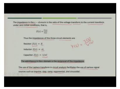
Now, when we talk about the impedance in s-domain so impedance would be nothing but the ratio of voltage Laplace transform and current Laplace transform under zero initial conditions. So we can write impedance  $Z(s) = \frac{V(s)}{I(s)}$ . So, the impedance of these three circuit elements which we discussed will become Z(s) = R for resistance, for inductive it will be Z(s) = sL, for capacitor the Z(s) = 1/sC.
