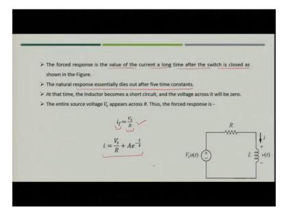
Now, what would be the forced response? Forced response is the value of the current a long time after the switch is closed. So, when you will see the circuit the natural response essentially dies out after 5 time constants. So, what will happen? At steady state condition say time t tends to infinity what will happen that the inductor will act as a short circuit.
