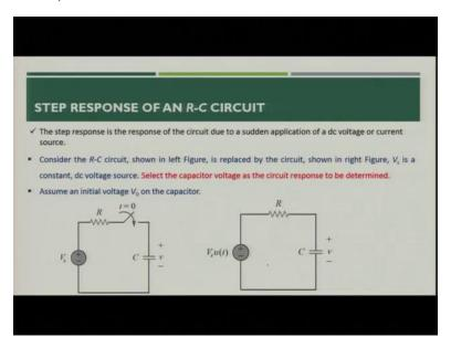
So, now let us recap what we discussed in the last class. We said that when time t is equal to 0 the circuit is closed then this particular phenomenon can be equivalently represented as a voltage source with a step function combined and then the RC circuit.
