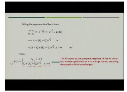
Now, let us see if the source voltage  $V_s > V_0$ . The plot would look like as shown in the figure. If you see this particular equation at time t is equal to 0 the value will start increasing. So, when we plot the curve for t less than just before 0 we will keep the value of voltage as  $V_0$ . So, what we have done? We have kept the voltage as  $V_0$  and then after that it is  $(V_0 - V_s)e^{-\frac{t}{\tau}}$ .
