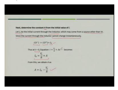
Now, next we have to find the value of constant A. Let us assume  $I_0$  is the initial current which will be flowing through the conductor that means at time t is equal to 0 minus means the time just before the application of the switch means the circuit is switched on and voltage source is applied.
