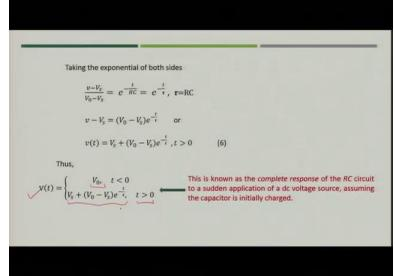
And we found that the equation for the RC circuit which we are seeing in the figure was derived with the help of mesh equations. Now, when we derived, we came to know  $V_0$  will remain same when time t < 0 and when time t > 0 this value can be calculated with the help of this expression that is  $V_s + (V_0 - V_s)e^{-\frac{t}{\tau}}$ . So, this is what we discussed in our previous lecture.
