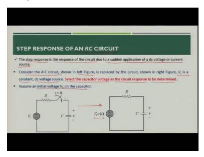
So, now let us start the step response of a circuit because we have understood the basic functions which are called as singularity functions. The unit step function is very important because when we talk about the step response of an RC circuit, we will say that when we apply the voltage that means, we are talking about the step input to the source step input to the circuit.
