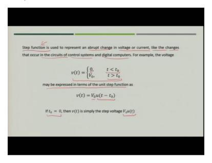
Now, step function is used to represent an abrupt change in voltage or current. So, whenever you apply voltage or current to the circuit through some switching arrangement it is nothing but you suddenly apply the source to the circuit and it is represented with the help of the unit step function because the value of voltage will not be 1 it will be some value.
