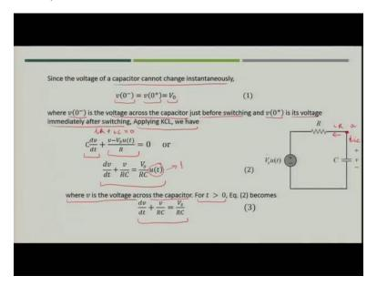
So, when you will say that it is charged with some voltage  $V_0$  we can say that at time  $t=0^-$  or at time t=0+, voltage will remain same as  $V_0$  because capacitor cannot change the voltage instantaneously. So, at t=0- the voltage across capacitor just before the switching happens and 0 plus is the voltage immediately after the switching happened. Now, if you apply KCL in this circuit what do you get?
